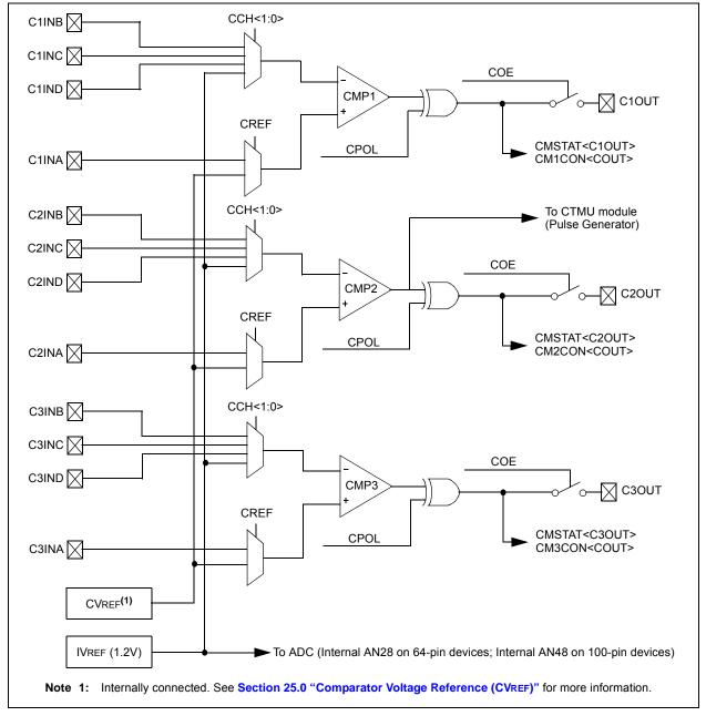
FIGURE 24-1: COMPARATOR BLOCK DIAGRAM
