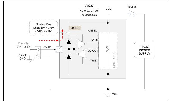
FIGURE 2-7: PIC32 5V TOLERANT PIN ARCHITECTURE EXAMPLE
