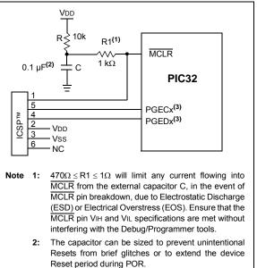
No pull-ups or bypass capacitors are allowed on active debug/program PGECx/PGEDx pins.
