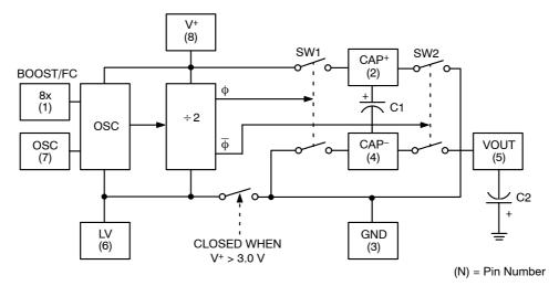
Figure 15. CAT660 Block Diagram
