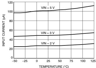
Figure 5. Supply Current vs. Temperature (No Load)
