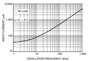
Figure 12. Supply Current vs. Oscillator Frequency
