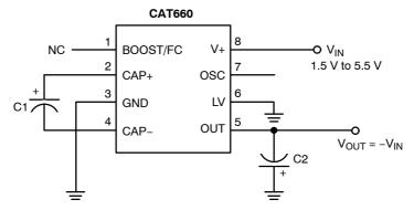
Figure 18. Voltage Inverter
