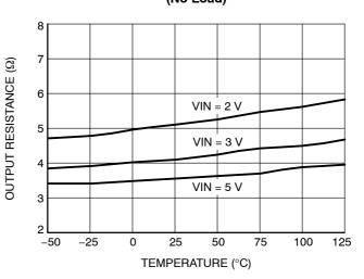
Figure 7. Output Resistance vs. Temperature (50  $\Omega$  Load)
