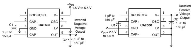
Figure 1. Voltage Inverter
