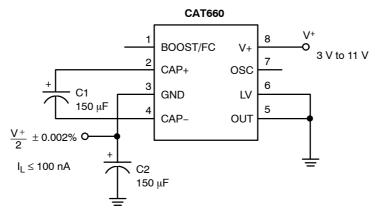
Figure 20. Precision Voltage Divider (Load ≤ 100 nA)
