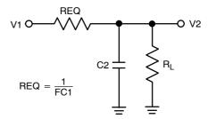
Figure 14. Switched-Capacitor Equivalent Circuit
