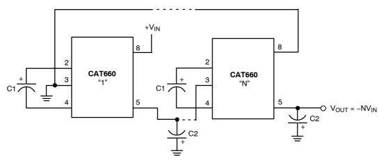
Figure 22. Cascading to Increase Output Voltage
