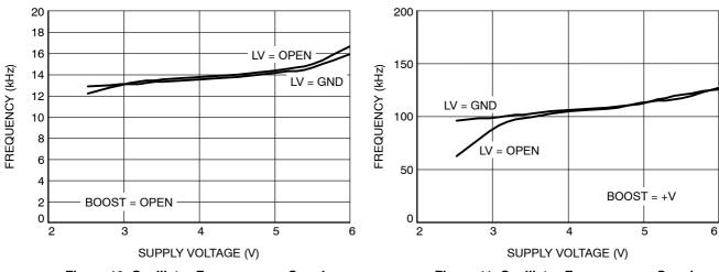
Figure 10. Oscillator Frequency vs. Supply Voltage
