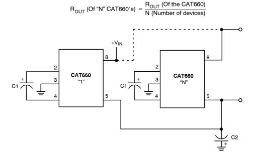
Figure 23. Paralleling Devices Reduce Output Resistance
