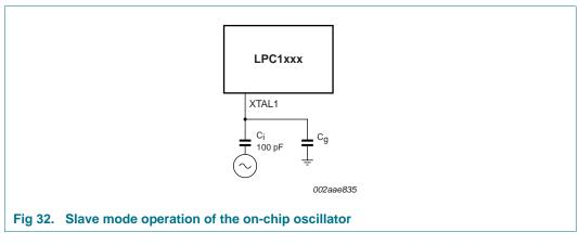
In slave mode the input clock signal should be coupled by means of a capacitor of 100 pF (Figure 32), with an amplitude between 200 mV(RMS) and 1000 mV(RMS). This corresponds to a square wave signal with a signal swing of between 280 mV and 1.4 V. The XTALOUT pin in this configuration can be left unconnected.
