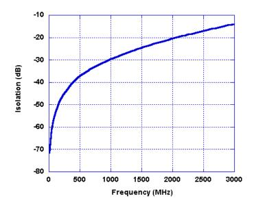
Figure 13. Isolation – Output to Output
