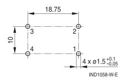
Tolerances to ISO 2768-cl / ISO 8015. Size ISO 14405 © All dimensions in mm
