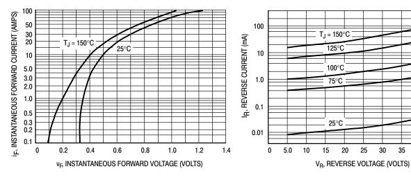
Figure 1. Typical Forward Voltage
