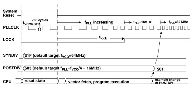
Figure 7-31. Startup of clock system after Reset
