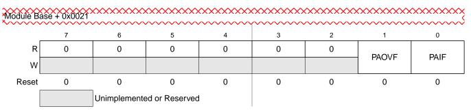
Figure 14-25. Pulse Accumulator Flag Register (PAFLG)
