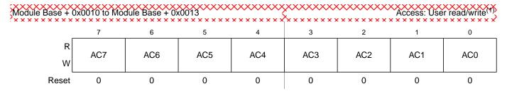
Figure 8-20. MSCAN Identifier Acceptance Registers (First Bank) — CANIDAR0-CANIDAR3
