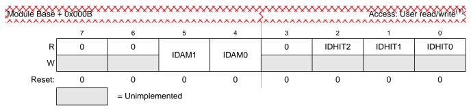
Figure 8-15. MSCAN Identifier Acceptance Control Register (CANIDAC)
