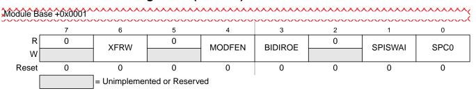
Figure 12-4. SPI Control Register 2 (SPICR2)
