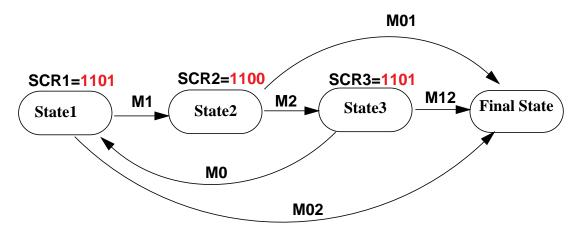
On simultaneous matches the lowest channel number has priority so with this configuration the forking from State1 has the peculiar effect that a simultaneous match0/match1 transitions to final state but a simultaneous match2/match1transitions to state2.
