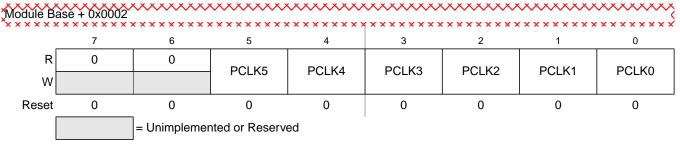
Figure 10-5. PWM Clock Select Register (PWMCLK)
