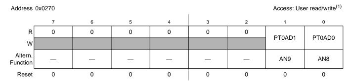
Figure 2-55. Port AD Data Register (PT0AD)
