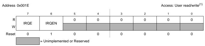
Figure 2-12. IRQ Control Register (IRQCR)
