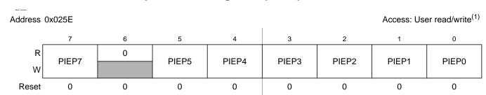
Figure 2-44. Port P Interrupt Enable Register (PIEP)
