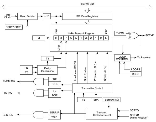
Figure 11-16. Transmitter Block Diagram
