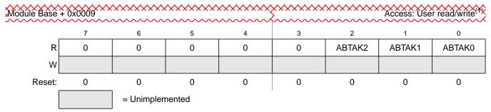
Figure 8-13. MSCAN Transmitter Message Abort Acknowledge Register (CANTAAK)
