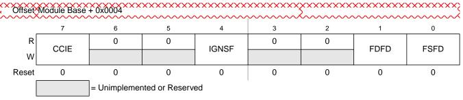
Figure 13-9. Flash Configuration Register (FCNFG)
