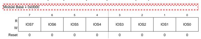
Figure 14-6. Timer Input Capture/Output Compare Select (TIOS)
