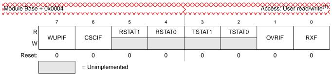
Figure 8-8. MSCAN Receiver Flag Register (CANRFLG)
