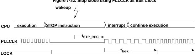
Figure 7-32. Stop Mode using PLLCLK as Bus Clock
