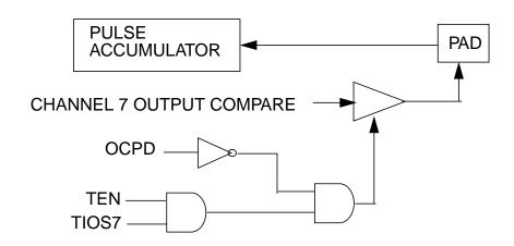
Figure 14-4. Channel 7 Output Compare/Pulse Accumulator Logic
