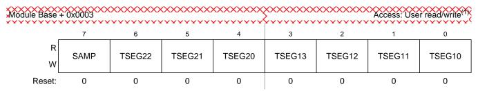
Figure 8-7. MSCAN Bus Timing Register 1 (CANBTR1)
