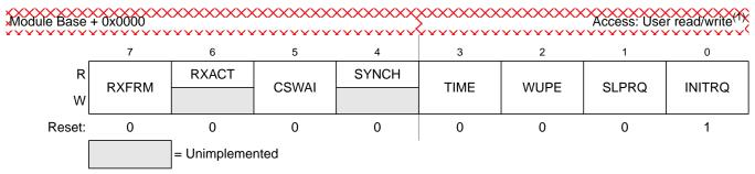
Figure 8-4. MSCAN Control Register 0 (CANCTL0)
