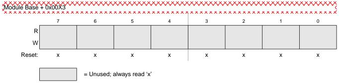
Figure 8-33. Identifier Register 3 — Standard Mapping
