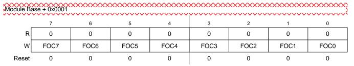
Figure 14-7. Timer Compare Force Register (CFORC)
