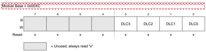
Figure 8-35. Data Length Register (DLR) — Extended Identifier Mapping
