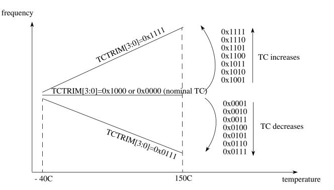
Figure 7-27. Influence of TCTRIM[3:0] on the Temperature Coefficient
