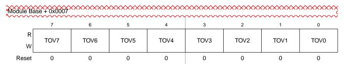
Figure 14-13. Timer Toggle On Overflow Register 1 (TTOV)
