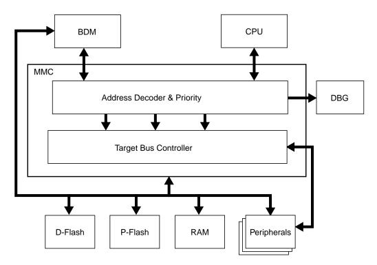
Figure 3-1. S12PMMC Block Diagram
