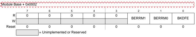
Figure 11-8. SCI Alternative Control Register 2 (SCIACR2)
