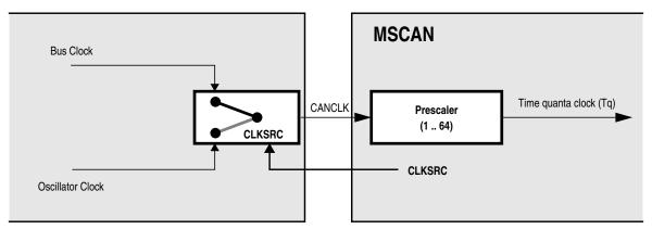
Figure 8-43. MSCAN Clocking Scheme
