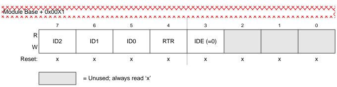
Figure 8-31. Identifier Register 1 — Standard Mapping
