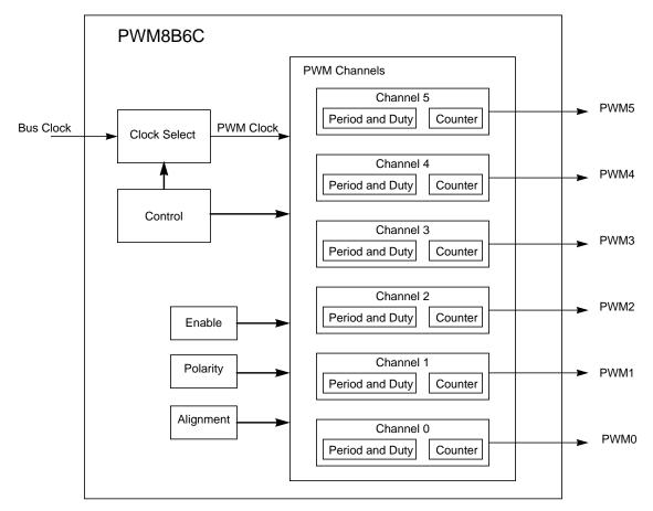
Figure 10-1. PWM8B6CV1 Block Diagram
