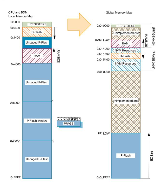
Figure 3-11. Implemented Global Address Mapping
