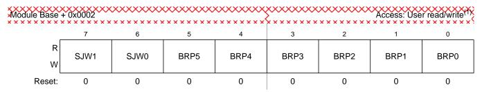
Figure 8-6. MSCAN Bus Timing Register 0 (CANBTR0)
