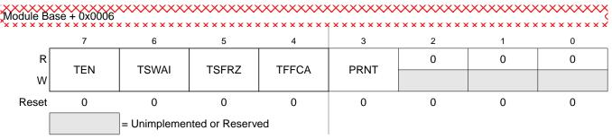
Figure 14-12. Timer System Control Register 1 (TSCR1)
