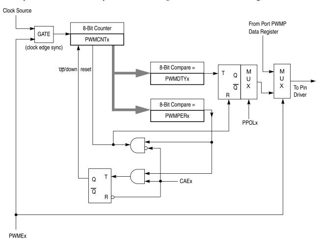
Figure 10-35. PWM Timer Channel Block Diagram
