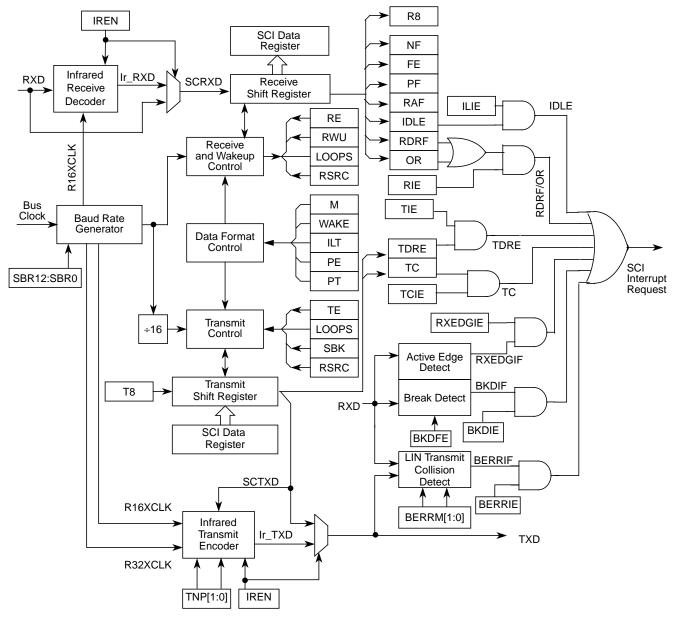
Figure 11-14. Detailed SCI Block Diagram
