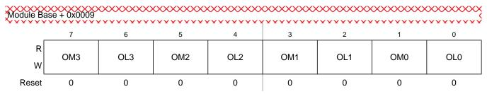
Figure 14-15. Timer Control Register 2 (TCTL2)
