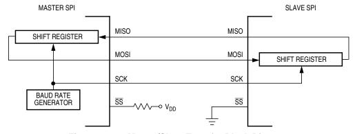
Figure 12-11. Master/Slave Transfer Block Diagram
