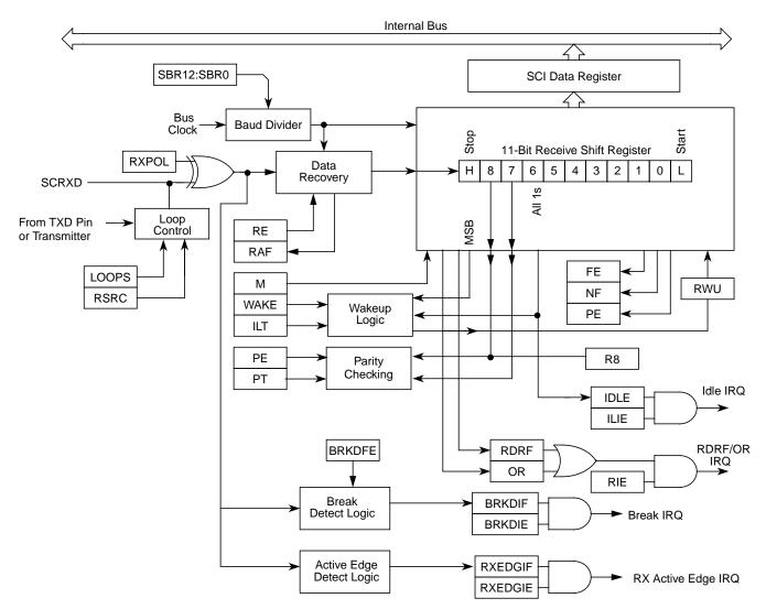
Figure 11-20. SCI Receiver Block Diagram
