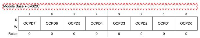
Figure 14-28. Ouput Compare Pin Disconnect Register (OCPD)
