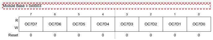
Figure 14-9. Output Compare 7 Data Register (OC7D)
