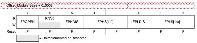
Figure 13-13. Flash Protection Register (FPROT)
