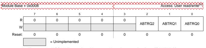
Figure 8-12. MSCAN Transmitter Message Abort Request Register (CANTARQ)
