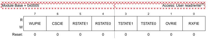
Figure 8-9. MSCAN Receiver Interrupt Enable Register (CANRIER)
