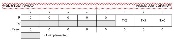
Figure 8-14. MSCAN Transmit Buffer Selection Register (CANTBSEL)
