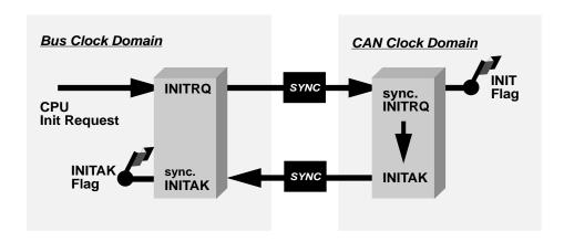
Figure 8-45. Initialization Request/Acknowledge Cycle
