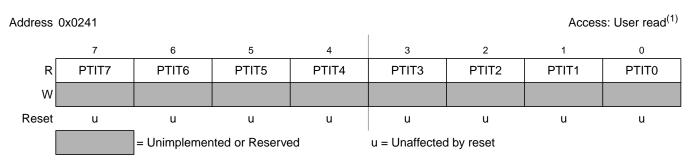
Figure 2-15. Port T Input Register (PTIT)
