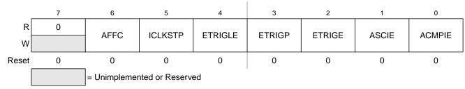
Figure 9-5. ATD Control Register 2 (ATDCTL2)
