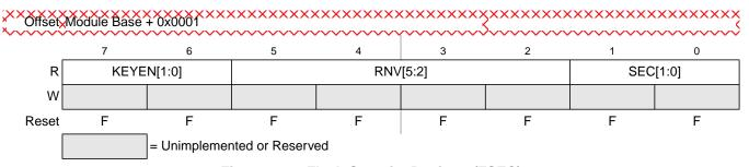
Figure 13-6. Flash Security Register (FSEC)
