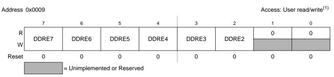
Figure 2-7. Port E Data Direction Register (DDRE)
