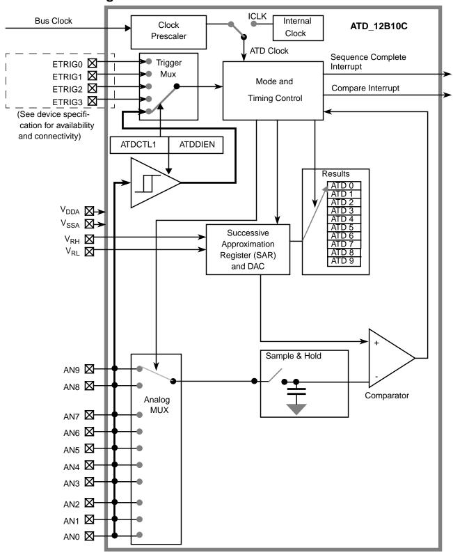
Figure 9-1. ADC12B10C Block Diagram
