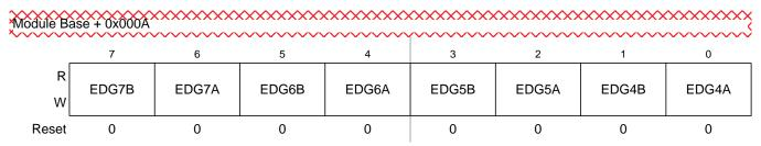
Figure 14-16. Timer Control Register 3 (TCTL3)
