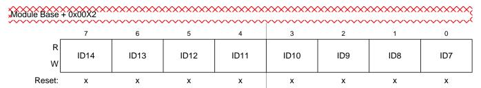
Figure 8-28. Identifier Register 2 (IDR2) — Extended Identifier Mapping
