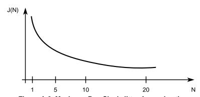
Figure A-3. Maximum Bus Clock Jitter Approximation
