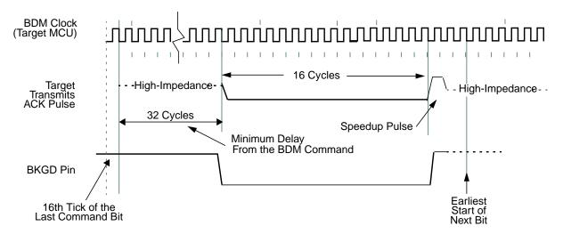
Figure 5-10. Target Acknowledge Pulse (ACK)
