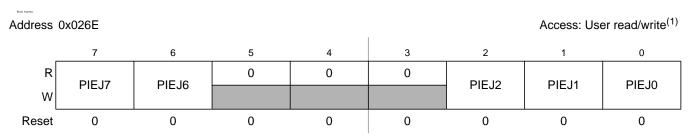
Figure 2-53. Port J Interrupt Enable Register (PIEJ)
