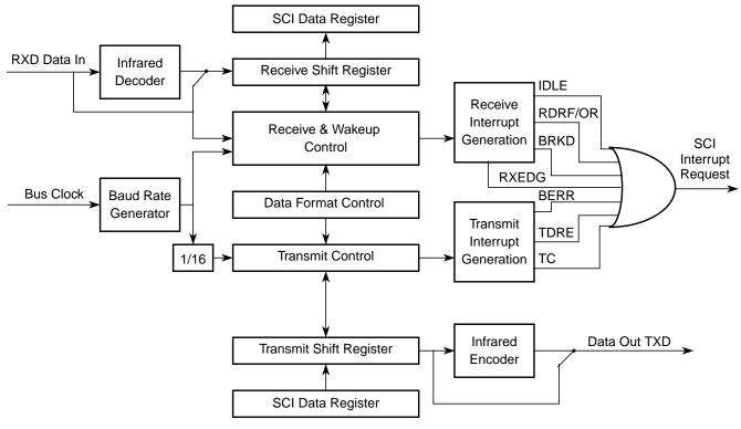
Figure 11-1. SCI Block Diagram
