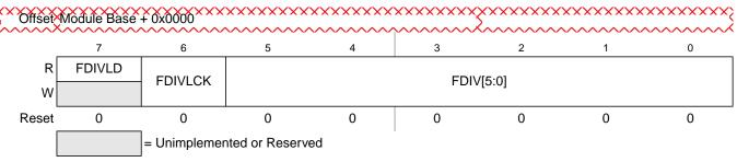
Figure 13-5. Flash Clock Divider Register (FCLKDIV)
