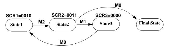
Scenario 10b shows the case that after M2 then M1 must occur before M0. Starting from a particular point in code, event M2 must always be followed by M1 before M0. If after any M2, event M0 occurs before M1 then a trigger is generated.
