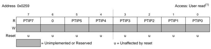
Figure 2-39. Port P Input Register (PTIP)
