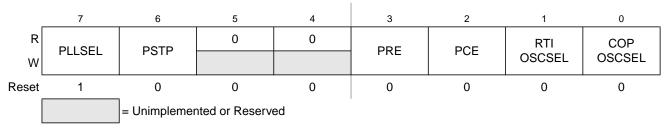
Figure 7-9. S12CPMU Clock Select Register (CPMUCLKS)
