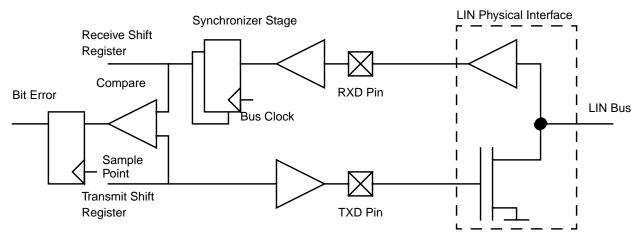
Figure 11-18. Collision Detect Principle
