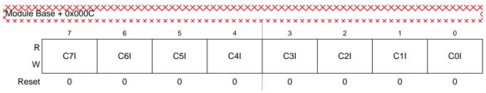
Figure 14-18. Timer Interrupt Enable Register (TIE)
