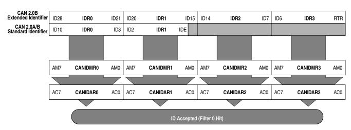
Figure 8-40. 32-bit Maskable Identifier Acceptance Filter
