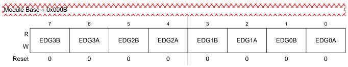
Figure 14-17. Timer Control Register 4 (TCTL4)
