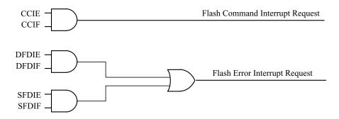
Figure 13-27. Flash Module Interrupts Implementation
