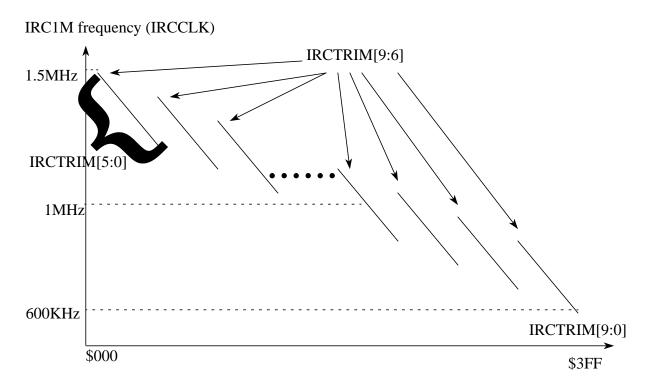
Figure 7-26. IRC1M Frequency Trimming Diagram
