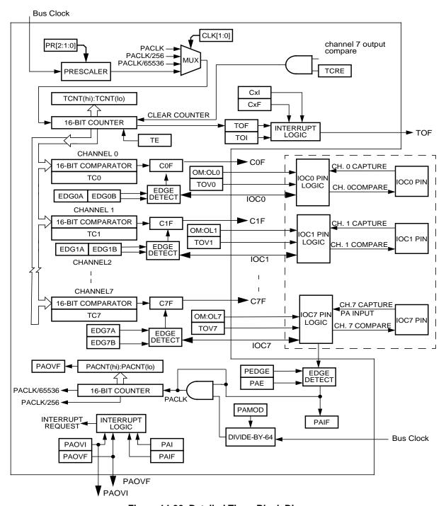
Figure 14-30. Detailed Timer Block Diagram
