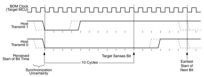
Figure 5-7. BDM Host-to-Target Serial Bit Timing
