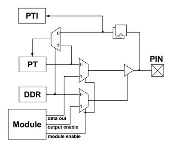
Figure 2-64. Illustration of I/O pin functionality
