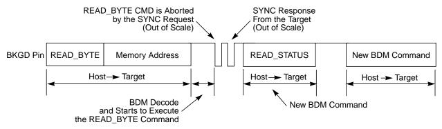
Figure 5-12. ACK Abort Procedure at the Command Level
