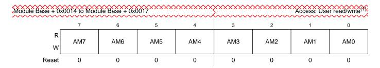
Figure 8-22. MSCAN Identifier Mask Registers (First Bank) — CANIDMR0-CANIDMR3
