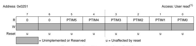
Figure 2-31. Port M Input Register (PTIM)
