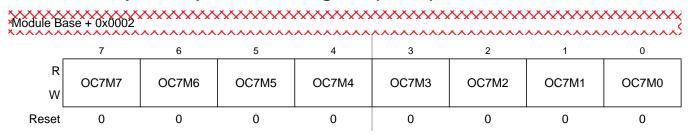
Figure 14-8. Output Compare 7 Mask Register (OC7M)
