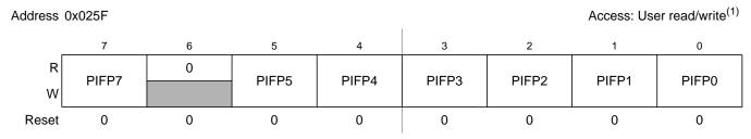
Figure 2-45. Port P Interrupt Flag Register (PIFP)
