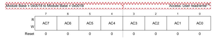
Figure 8-21. MSCAN Identifier Acceptance Registers (Second Bank) — CANIDAR4-CANIDAR7
