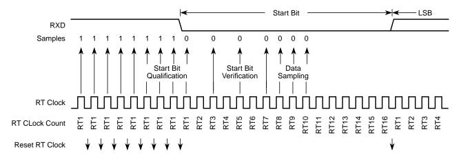
Figure 11-21. Receiver Data Sampling
