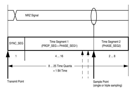
Figure 8-44. Segments within the Bit Time
