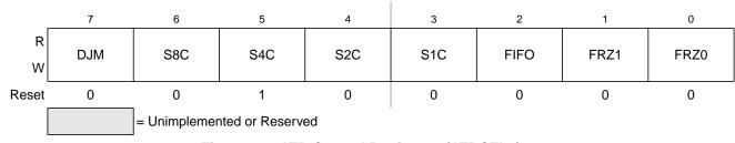
Figure 9-6. ATD Control Register 3 (ATDCTL3)
