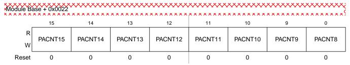
Figure 14-26. Pulse Accumulator Count Register High (PACNTH)
