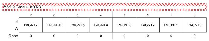
Figure 14-27. Pulse Accumulator Count Register Low (PACNTL)
