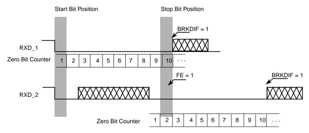
Figure 11-17. Break Detection if BRKDFE = 1 (M = 0)
