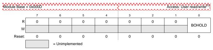
Figure 8-17. MSCAN Miscellaneous Register (CANMISC)
