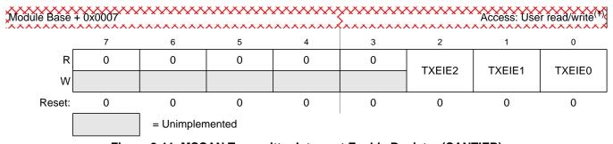
Figure 8-11. MSCAN Transmitter Interrupt Enable Register (CANTIER)
