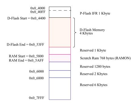
Figure 13-3. D-Flash and Memory Controller Resource Memory Map
