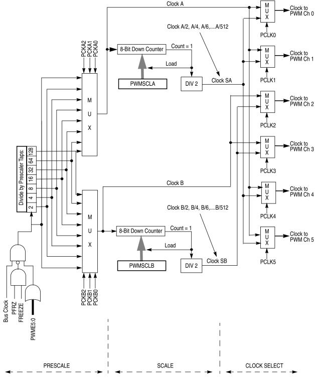
Figure 10-34. PWM Clock Select Block Diagram
