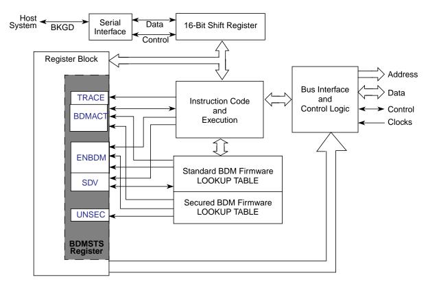
Figure 5-1. BDM Block Diagram
