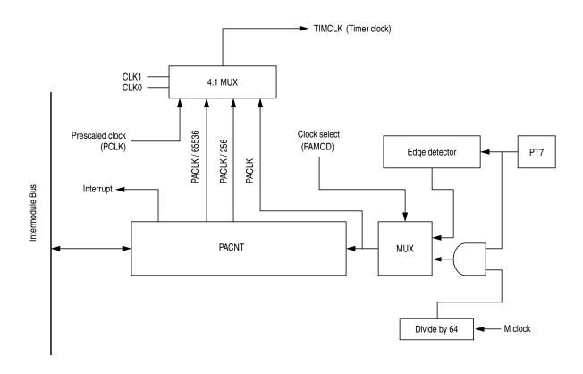
Figure 14-2. 16-Bit Pulse Accumulator Block Diagram
