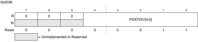
Figure 7-6. S12CPMU Post Divider Register (CPMUPOSTDIV)
