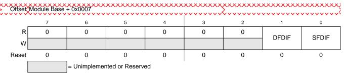
Figure 13-12. Flash Error Status Register (FERSTAT)
