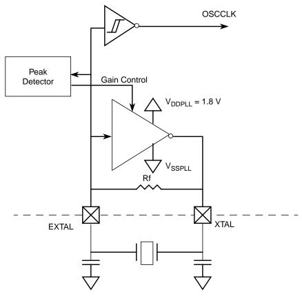
Figure 7-2. OSCLCP Block Diagram
