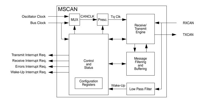
Figure 8-1. MSCAN Block Diagram
