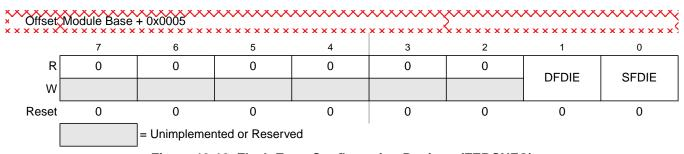
Figure 13-10. Flash Error Configuration Register (FERCNFG)
