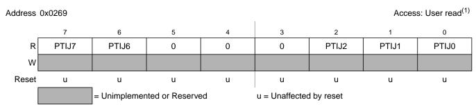
Figure 2-48. Port J Input Register (PTIJ)
