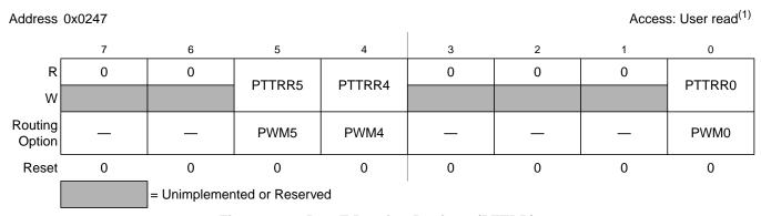
Figure 2-21. Port T Routing Register (PTTRR)
