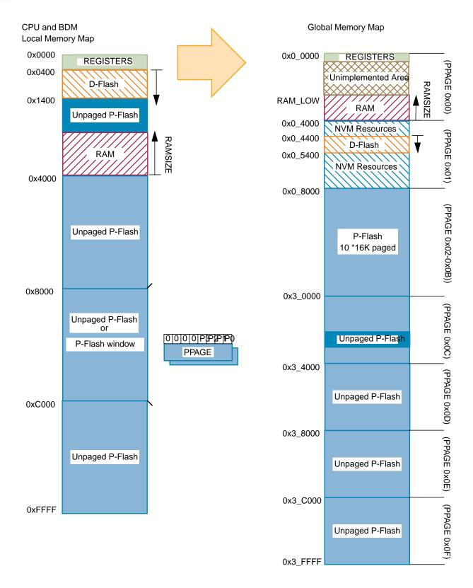
Figure 3-10. Local to Global Address Mapping
