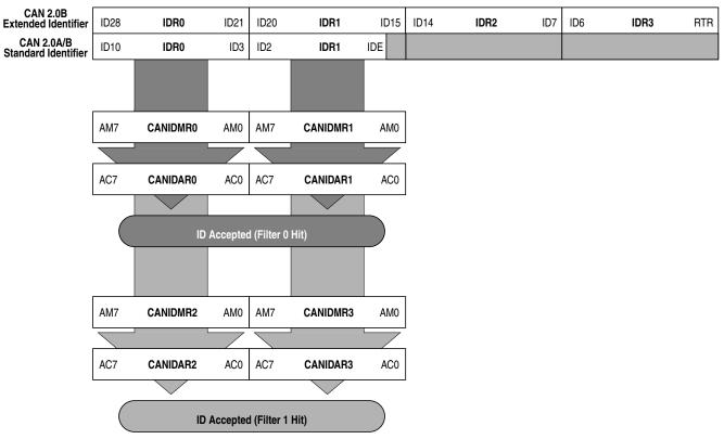
Figure 8-41. 16-bit Maskable Identifier Acceptance Filters
