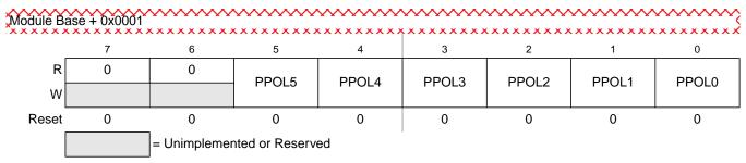
Figure 10-4. PWM Polarity Register (PWMPOL)
