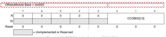
Figure 13-7. FCCOB Index Register (FCCOBIX)
