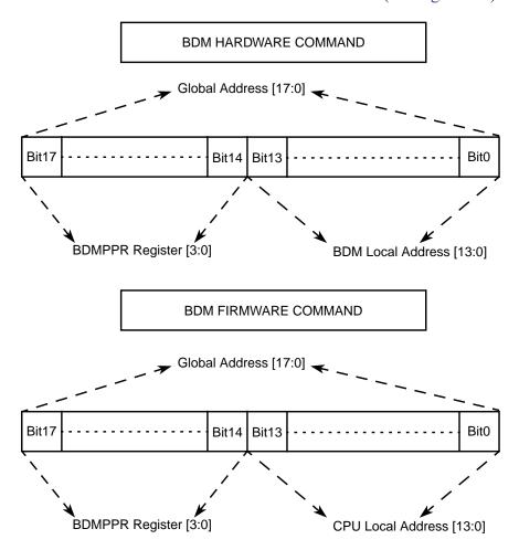
Figure 3-9. BDMPPR Address Mapping
