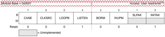
Figure 8-5. MSCAN Control Register 1 (CANCTL1)
