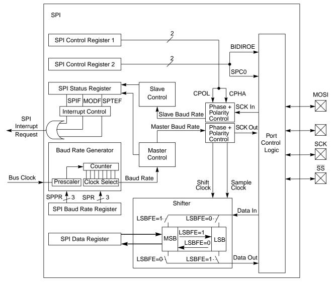
Figure 12-1. SPI Block Diagram
