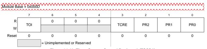
Figure 14-19. Timer System Control Register 2 (TSCR2)
