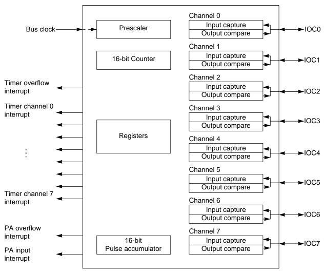
Figure 14-1. TIM16B8CV2 Block Diagram
