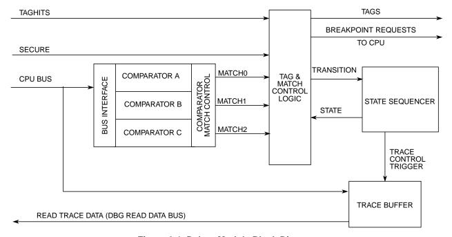
Figure 6-1. Debug Module Block Diagram
