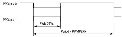
Figure 10-36. PWM Left Aligned Output Waveform
