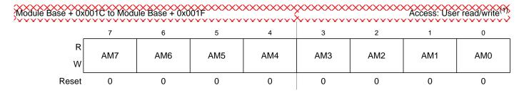
Figure 8-23. MSCAN Identifier Mask Registers (Second Bank) — CANIDMR4-CANIDMR7
