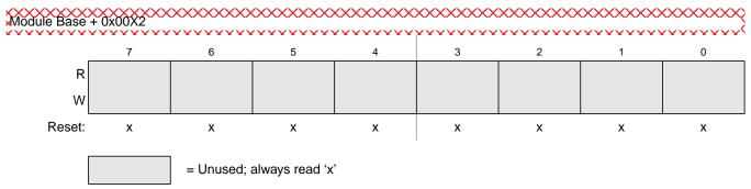
Figure 8-32. Identifier Register 2 — Standard Mapping
