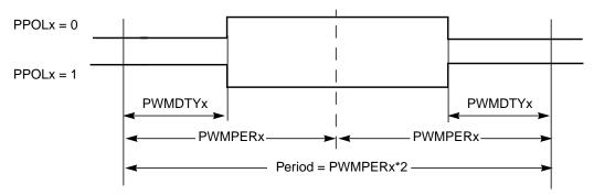
Figure 10-38. PWM Center Aligned Output Waveform
