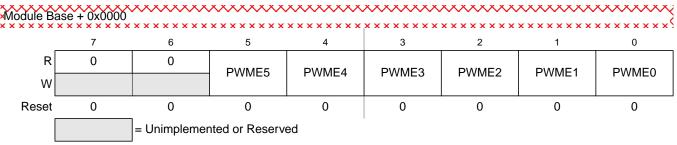
Figure 10-3. PWM Enable Register (PWME)
