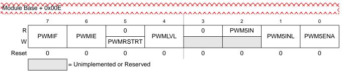
Figure 10-33. PWM Shutdown Register (PWMSDN)
