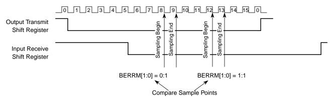
Figure 11-19. Timing Diagram Bit Error Detection
