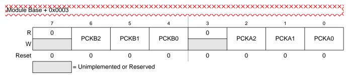
Figure 10-6. PWM Prescaler Clock Select Register (PWMPRCLK)
