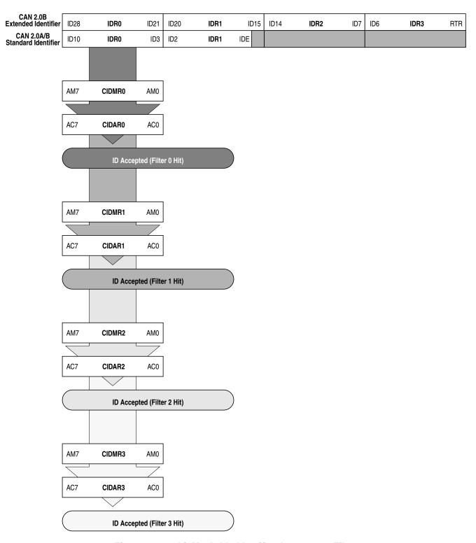
Figure 8-42. 8-bit Maskable Identifier Acceptance Filters
