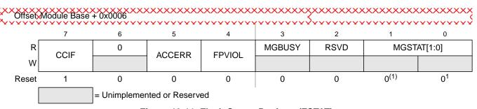
Figure 13-11. Flash Status Register (FSTAT)
