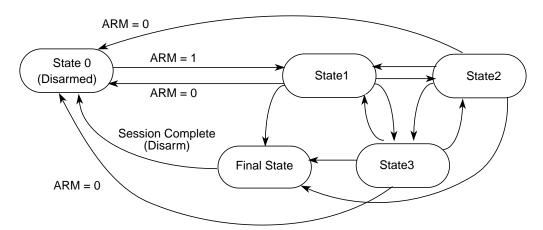
Figure 6-24. State Sequencer Diagram
