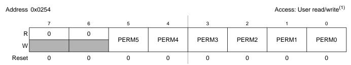
Figure 2-34. Port M Pull Device Enable Register (PERM)
