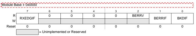
Figure 11-6. SCI Alternative Status Register 1 (SCIASR1)
