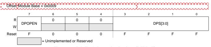
Figure 13-15. D-Flash Protection Register (DFPROT)
