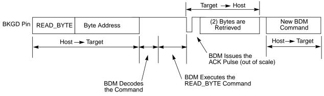
Figure 5-11. Handshake Protocol at Command Level
