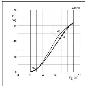
$V_{CB}$  = 40 V; class-C;  $t_p$  = 100  $\mu$ s;  $\delta$  = 10%.
