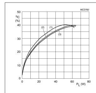
$V_{CB}$  = 40 V; class-C;  $t_p$  = 100  $\mu s; \, \delta$  = 10%.
