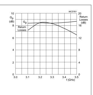
$V_{CB}$  = 40 V; class-C;  $P_L$  = 50 W;  $t_p$  = 100  $\mu s;$   $\delta$  = 10%.
