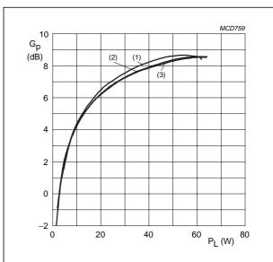
$V_{CB}$  = 40 V; class-C;  $P_{L}$  = 50 W;  $t_{p}$  = 100  $\mu$ s;  $\delta$  = 10%.
