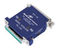
The RS-232 port uses a female DB-25 type of connector with pins 2 (TD input) and 3 (RD output) supported. Protective Ground (pin 1) and Signal Ground (pin 7) are also connected. The RS-422 port uses a male DB-25 type of connector with the Send Data outputs on pins 2 and 14, and the Receive Data inputs on pins 5 and 17. Protective Ground (pin 1) and Signal Ground (pin 7) are connected through to the RS-232 connector.
