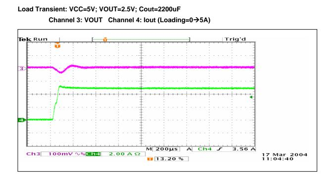
Load Transient: VCC=5V; VOUT=2.5V; Cout=2200uF Channel 3: VOUT Channel 4: lout (Loading=5→0A)
