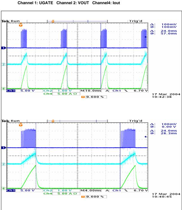
Short Hiccup: VCC=5V; VOUT=2.5V; Cout=2200uF with R=0.1(ohm) load.
