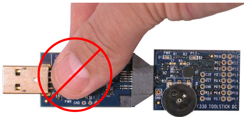
Figure 2. Improper Method of Holding the ToolStick
