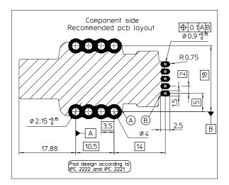
(Layout example with 4 jumpers in parallel)
