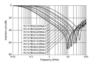
Common Mode Insertion Loss-Frequency Characteristics
