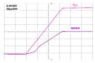
FIGURE 22. POWER-ON START-UP IN VOLTAGE DIVIDER MODE
