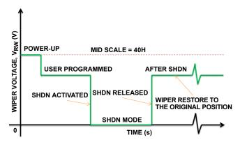
FIGURE 26. SHUTDOWN MODE WIPER RESPONSE
