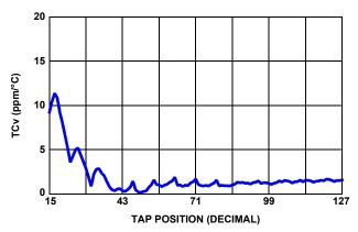
FIGURE 17. 100k $\Omega$  TCv vs TAP POSITION, V<sub>CC</sub> = 3.3V
