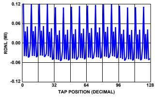
FIGURE 7. 10k $\Omega$  RDNL vs TAP POSITION, V<sub>CC</sub> = 3.3V, +25°C
