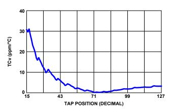
FIGURE 14.  $50k\Omega$  TCv vs TAP POSITION,  $V_{CC} = 3.3V$
