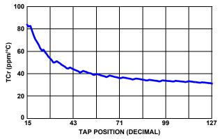
FIGURE 16.  $50k\Omega$  TCr vs TAP POSITION,  $V_{CC} = 3.3V$
