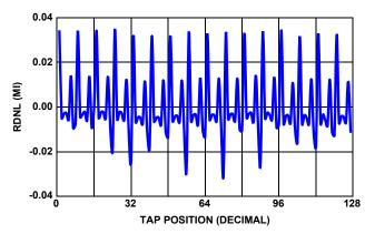
FIGURE 8.  $50 \text{k}\Omega$  RDNL vs TAP POSITION,  $V_{\text{CC}}$  = 3.3V, +25°C
