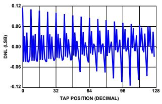
FIGURE 3. 10k $\Omega$  DNL vs TAP POSITION, V<sub>CC</sub> = 3.3V, +25 °C
