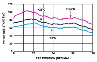
FIGURE 12.  $50 \text{k}\Omega$  WIPER RESISTANCE vs TAP POSITION,  $V_{\text{CC}}$  = 3.3 V
