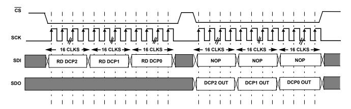
FIGURE 32. DAISY CHAIN READ SEQUENCE OF N =  $3\ DCP$
