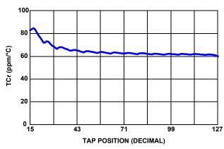
FIGURE 18. 100k $\Omega$  TCr vs TAP POSITION, V<sub>CC</sub> = 3.3V
