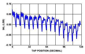
FIGURE 5. 10k $\Omega$  INL vs TAP POSITION, V<sub>CC</sub> = 3.3V, +25 °C
