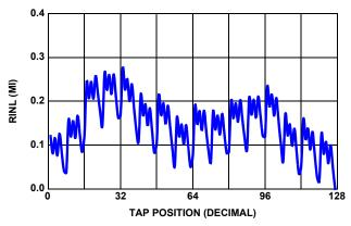
FIGURE 9. 10k $\Omega$  RINL vs TAP POSITION, V<sub>CC</sub> = 3.3V, +25 °C
