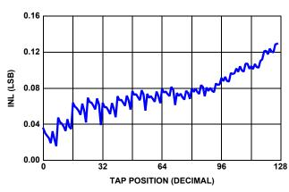
FIGURE 6.  $50k\Omega$  INL vs TAP POSITION,  $V_{CC}$  = 3.3V, +25°C
