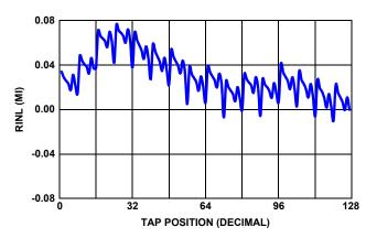
FIGURE 10.  $50k\Omega$  RINL vs TAP POSITION,  $V_{CC}$  = 3.3V, +25°C
