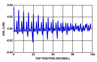
FIGURE 4.  $50k\Omega$  DNL vs TAP POSITION,  $V_{CC} = 3.3V$ ,  $+25\,^{\circ}C$
