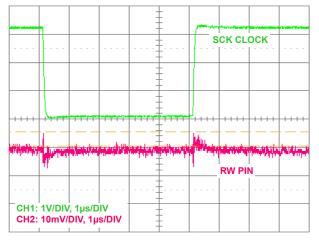
FIGURE 19. WIPER DIGITAL FEED-THROUGH
