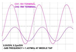
FIGURE 23. 10kΩ -3dB CUT OFF FREQUENCY
