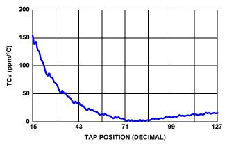
FIGURE 13. 10k $\Omega$  TCv vs TAP POSITION, V<sub>CC</sub> = 3.3V
