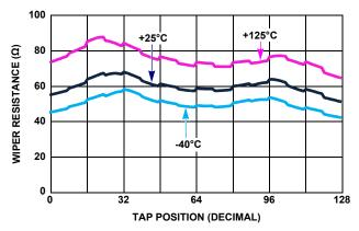
FIGURE 11.  $10k\Omega$  WIPER RESISTANCE vs TAP POSITION,  $V_{CC} = 3.3V$
