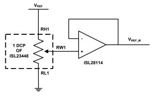
FIGURE 2. V<sub>REF</sub> ADJUSTMENT
