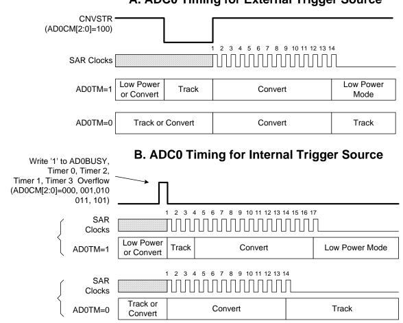
A. ADC0 Timing for External Trigger Source
