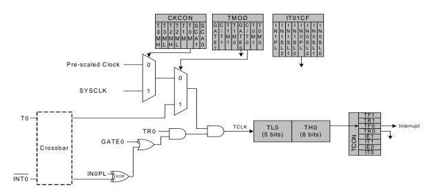
Figure 32.1. T0 Mode 0 Block Diagram
