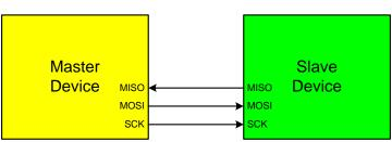
Figure 30.3. 3-Wire Single Master and 3-Wire Single Slave Mode Connection Diagram
