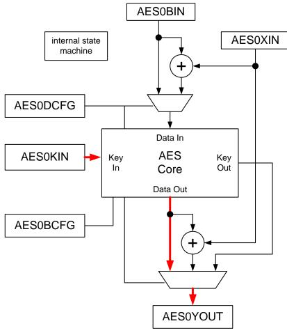
Figure 14.2. Key Inversion Data Flow
