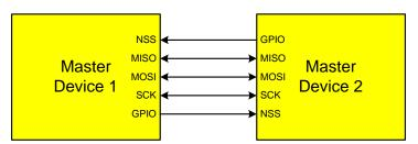
Figure 30.2. Multiple-Master Mode Connection Diagram
