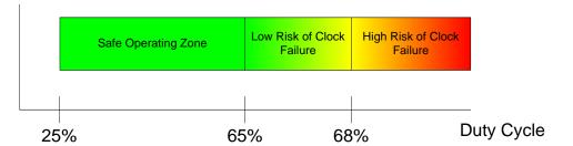
Figure 24.2. Interpreting Oscillation Robustness (Duty Cycle) Test Results
