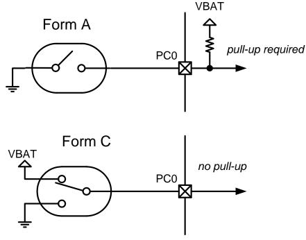
Figure 25.3. Reed Switch Configurations
