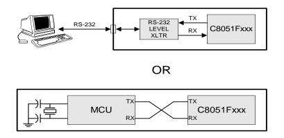
Figure 29.3. UART Interconnect Diagram
