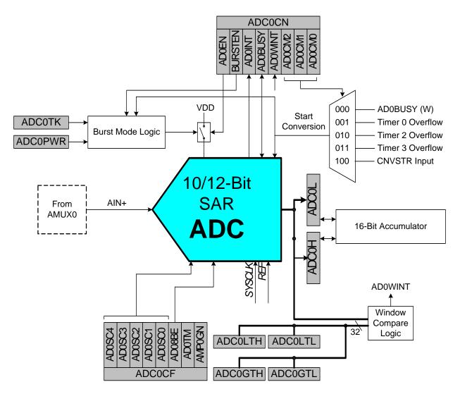
Figure 1.13. ADC0 Functional Block Diagram
