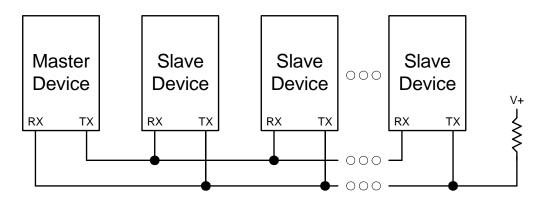
Figure 29.6. UART Multi-Processor Mode Interconnect Diagram
