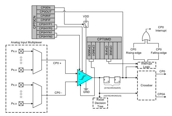
Figure 7.1. Comparator 0 Functional Block Diagram
