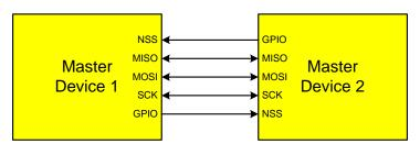
Figure 31.2. Multiple-Master Mode Connection Diagram
