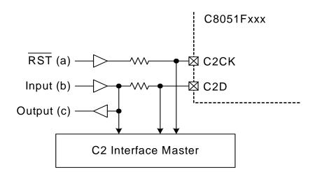
Figure 34.1. Typical C2 Pin Sharing
