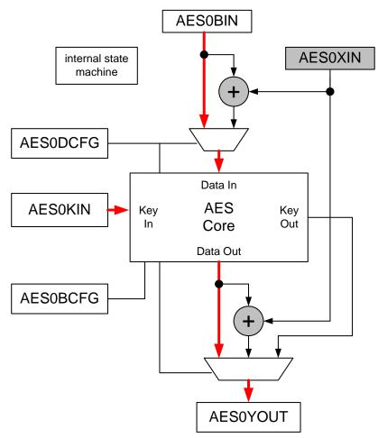
Figure 14.3. AES Block Cipher Data Flow
