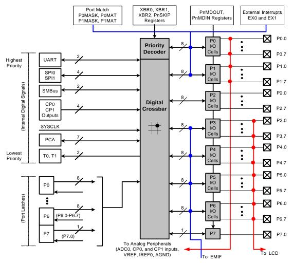
Figure 1.11. Port I/O Functional Block Diagram
