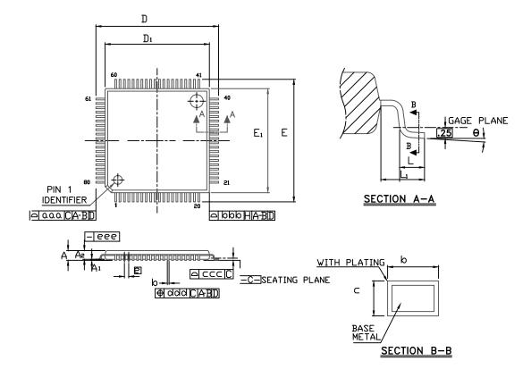
Figure 3.9. TQFP-80 Package Drawing
