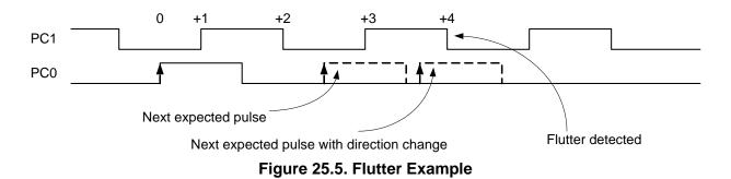
For example, flutter detected on the PC0 positive edge means that 4 edges (positive or negative) were detected on PC1 since the last PC0 positive edge. Each PC0 positive edge resets the flutter detection counter while either PC1 edge increments the counter. There are similar counters for all four edges.
