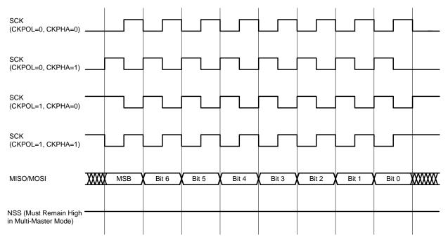
Figure 30.5. Master Mode Data/Clock Timing
