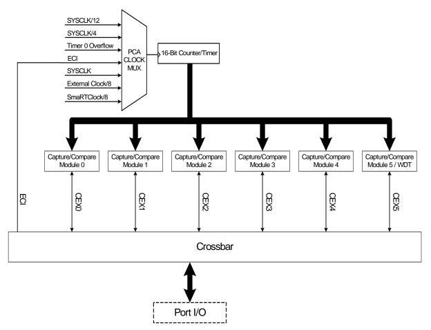
Figure 33.1. PCA Block Diagram
