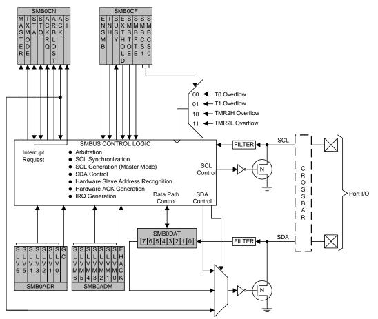
Figure 28.1. SMBus Block Diagram
