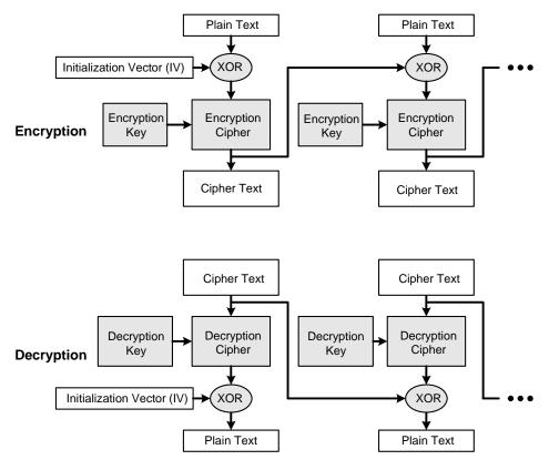
Figure 14.4. Cipher Block Chaining Mode
