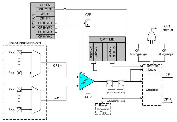
Figure 7.2. Comparator 1 Functional Block Diagram
