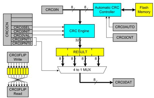
Figure 12.1. CRC0 Block Diagram
