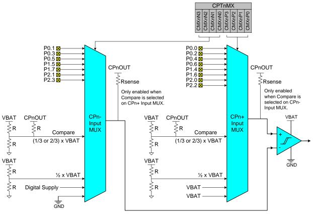
Figure 7.4. CPn Multiplexer Block Diagram
