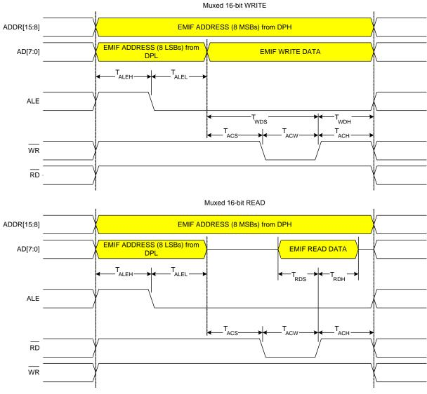
Figure 10.7. Multiplexed 16-bit MOVX Timing
