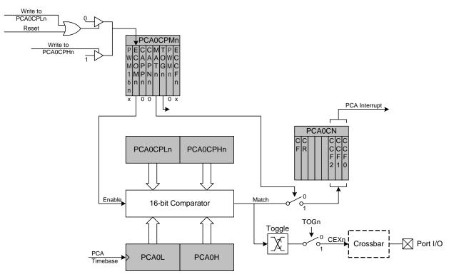
Figure 33.6. PCA High-Speed Output Mode Diagram
