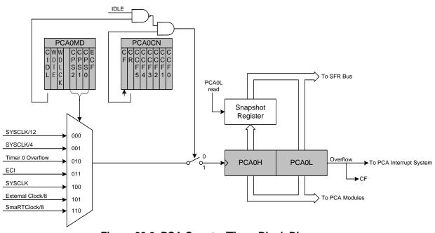
Figure 33.2. PCA Counter/Timer Block Diagram
