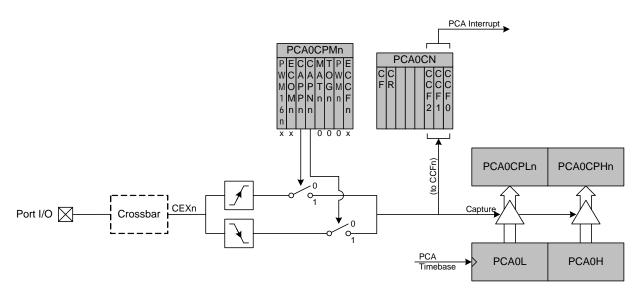
Figure 33.4. PCA Capture Mode Diagram
