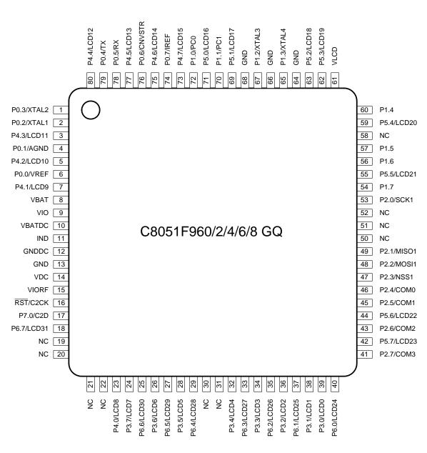
Figure 3.3. TQFP-80 Pinout Diagram (Top View)
