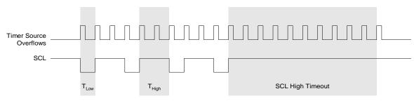
Figure 28.4. Typical SMBus SCL Generation
