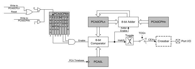
Figure 33.7. PCA Frequency Output Mode
