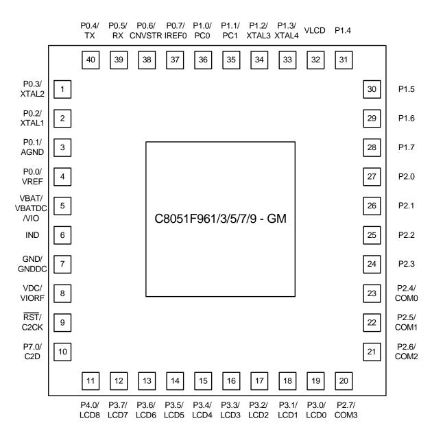
Figure 3.2. QFN-40 Pinout Diagram (Top View)
