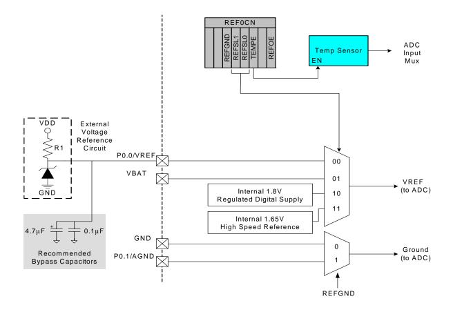
Figure 5.10. Voltage Reference Functional Block Diagram
