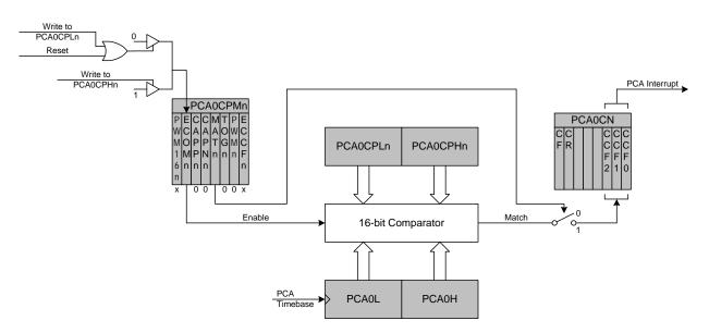
Figure 33.5. PCA Software Timer Mode Diagram
