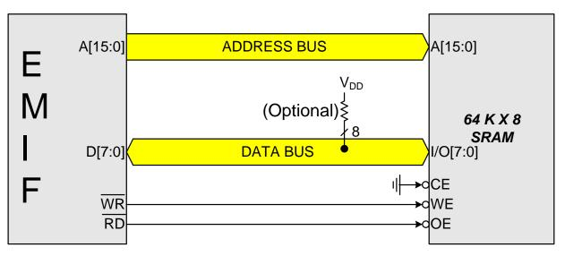
Figure 10.2. Non-multiplexed Configuration Example
