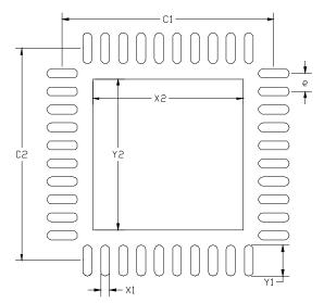
Figure 3.8. QFN-40 Landing Diagram
