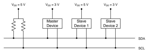
Figure 28.2. Typical SMBus Configuration
