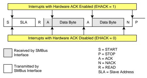
Figure 28.6. Typical Master Read Sequence
