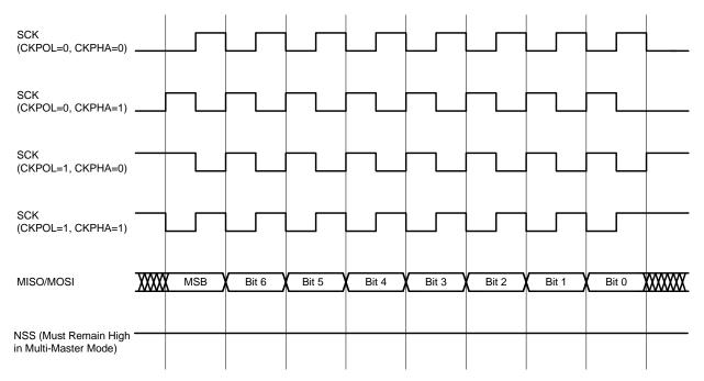
Figure 31.5. Master Mode Data/Clock Timing
