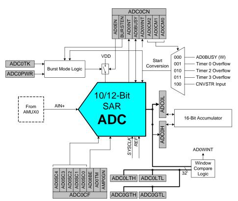
Figure 5.1. ADC0 Functional Block Diagram
