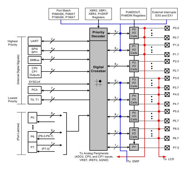
Figure 27.1. Port I/O Functional Block Diagram
