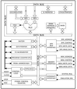
Figure 8.1. CIP-51 Block Diagram
