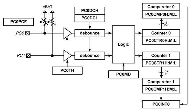
Figure 25.1. Pulse Counter Block Diagram
