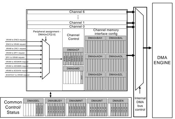
Figure 11.1. DMA0 Block Diagram
