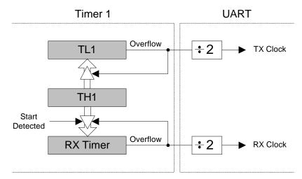
Figure 29.2. UART0 Baud Rate Logic
