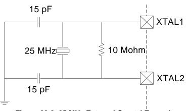
Figure 23.2. 25 MHz External Crystal Example
