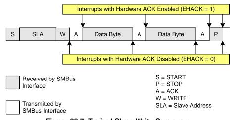
Figure 28.7. Typical Slave Write Sequence
