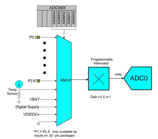
Figure 1.14. ADC0 Multiplexer Block Diagram
