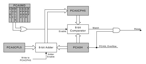
Figure 33.11. PCA Module 5 with Watchdog Timer Enabled
