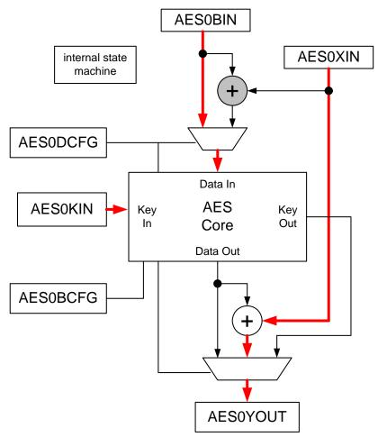
Figure 14.8. Counter Mode Data Flow
