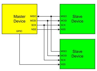
Figure 31.4. 4-Wire Single Master Mode and 4-Wire Slave Mode Connection Diagram
