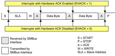
Figure 28.5. Typical Master Write Sequence
