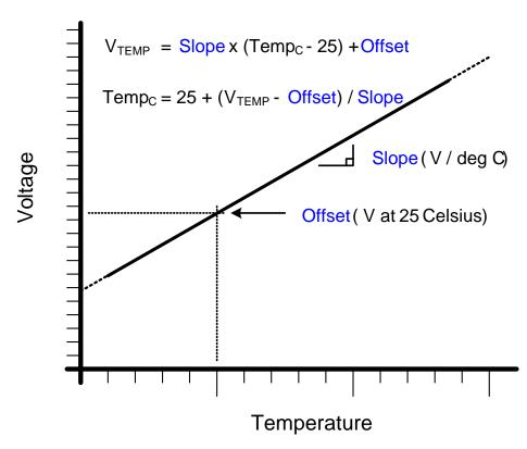
Figure 5.8. Temperature Sensor Transfer Function
