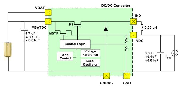
Figure 20.1 shows a block diagram of the buck converter.
