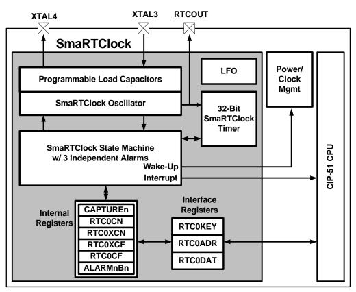
Figure 24.1. SmaRTClock Block Diagram
