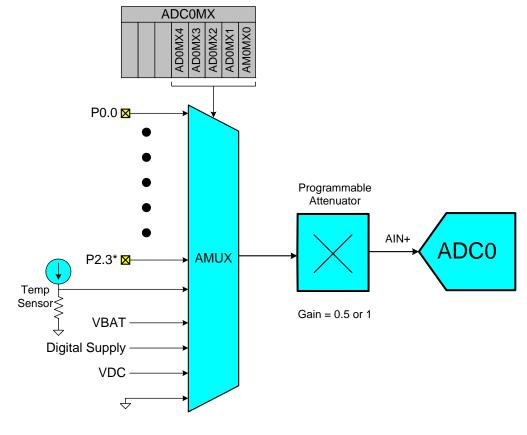
\*P1.0 – P1.3 are not available as analog inputs Figure 5.7. ADC0 Multiplexer Block Diagram
