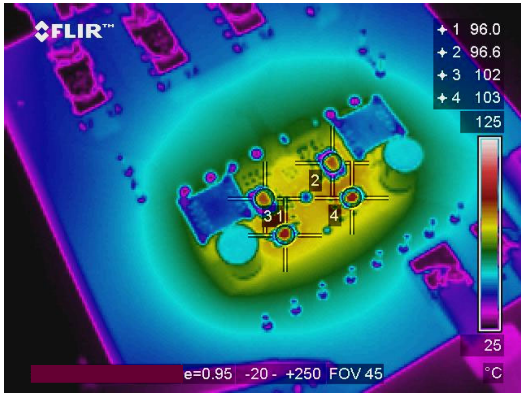
Fig.37: Thermal Image, Test Points 1, 2, 3, and 4 are Synchronous DirectFET for 2.5V output, Synchronous DirectFET for 1.8V output, Control DirectFET for 2.5V output, and Control DirectFET for 1.8V output, respectively.
