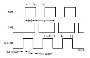
Figure 3. Timing Diagram RT/SYNC = 28.0k,  $t_P = 1\mu s$ ,  $V_{DIV} = 0V$
