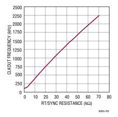
Figure 2. Switching Frequency vs RT/SYNC Resistance
