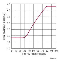
Figure 6. Peak Switch Current vs ILIM Resistor
