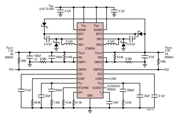
Figure 15. 3.3V and 1.2V Dual Step-Down Multi-Frequency Converter
