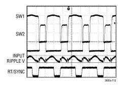
Figure 13. Dual 14.4V/8.5V, 14.4V/3.3V with 256° Phase
