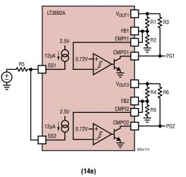
Figure 14. SS Pin Configurations
