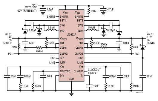
FMEA Fault Tolerant 3.3V/2A and 5V/2A Dual Converter
