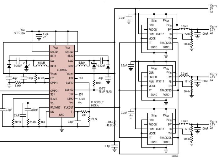
5V, 3.3V, 2.5V, 1.8V Synchronized Quad Output
