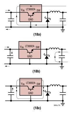
Figure 18. Subtracting the Current When the Switch Is On (18a) from the Current When the Switch Is Off (18b) Reveals the Path of the High Frequency Switching Current (18c). Keep this Loop Small. The Voltage on the SW and BST Traces Will Also Be Switched; Keep These Traces as Short as Possible. Finally, Make Sure the Circuit Is Shielded with a Local Ground Plane
