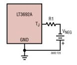
Figure 20. Circuit to Extend the  $T_{\rm J}$  Pin Operating Range
