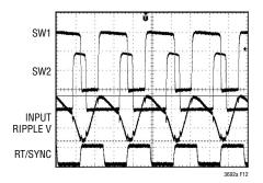
Figure 12. Dual 14.4V/8.5V, 14.4V/3.3V with 180° Phase
