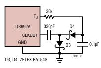
Figure 21. Circuit to Generate the Negative Voltage Rail to Extend the  $T_{\rm J}$  Pin Operating Range
