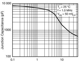
Reverse Voltage (V) Fig. 5 - Typical Junction Capacitance Per Diode
