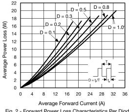
Fig. 2 - Forward Power Loss Characteristics Per Diode
