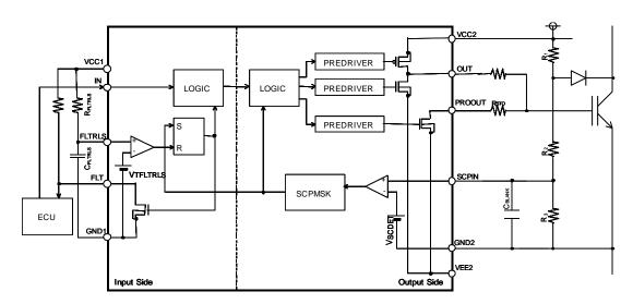
Figure 10. Block Diagram for DESAT
