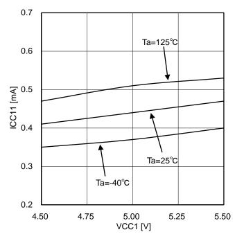
Figure 17. Input side circuit current (at OUT1=L)
