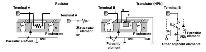
Figure 65. Pattern Diagram of Parasitic Element
