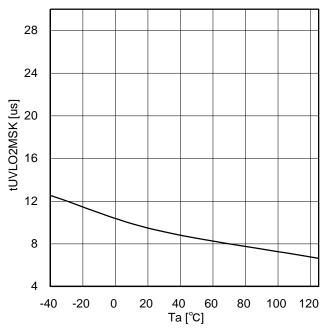
Figure 53. VCC2 UVLO mask time
