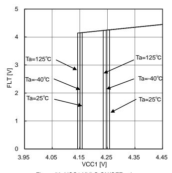
Figure 50. VCC1 UVLO ON/OFF voltage
