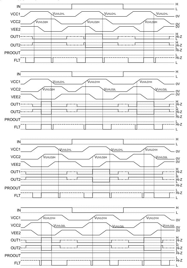
: Since the VCC2 to VEE2 pin voltage is low and the output MOS does not turn ON, the output pins become Hi-Z conditions.
