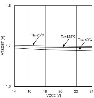
Figure 58. Thermal detection voltage
