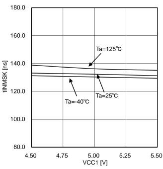
Figure 34. Logic (INA/INB) input mask time (Low pulse)
