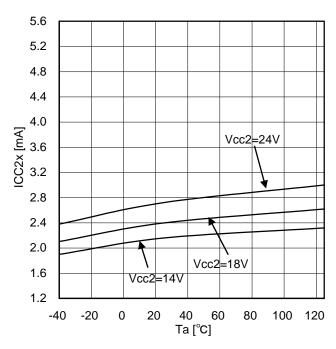
Figure 28. Output side circuit current (at OUT1=H)
