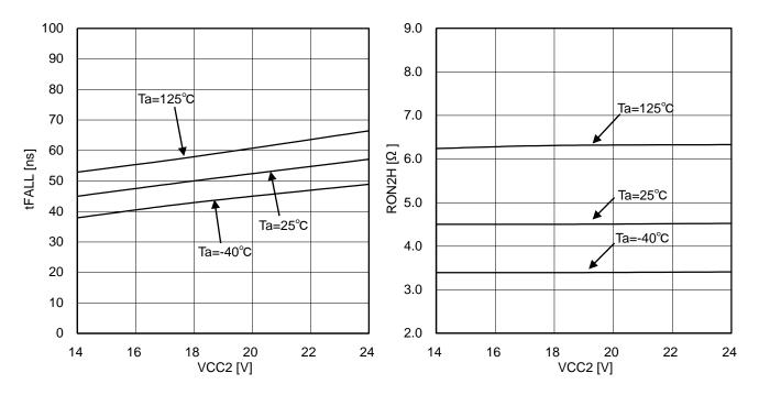
Figure 43. Fall time (10nF between OUT1-VEE2)
