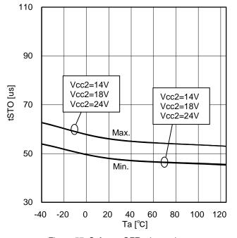
Figure 57. Soft turn OFF release time
