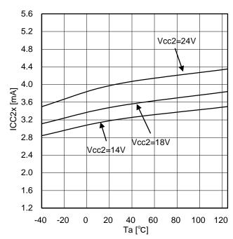
Figure 26. Output side circuit current (at OUT1=L)
