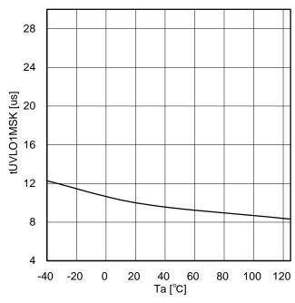
Figure 51. VCC1 UVLO mask time
