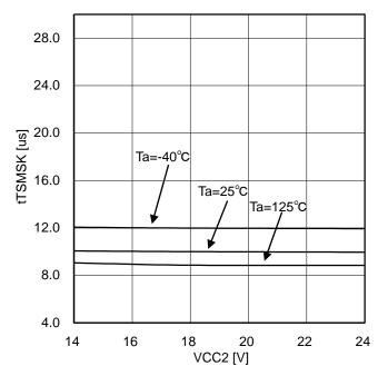
Figure 59. Thermal detection mask time
