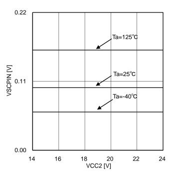
Figure 54. SCPIN input voltage (at ISCPIN=1mA)
