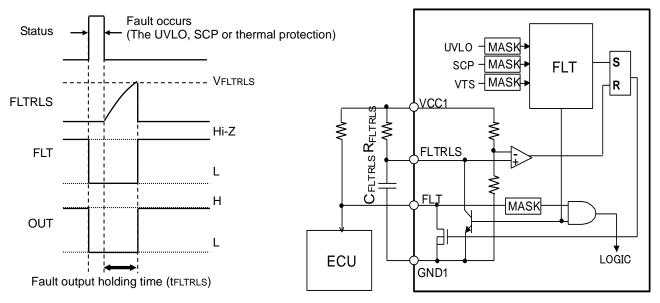
Figure 6. Fault Status Output Timing Chart
