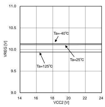
Figure 48. VREG output voltage
