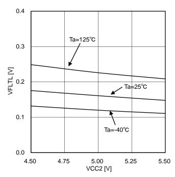
Figure 60. FLT output low voltage (IFLT=5mA)
