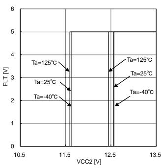
Figure 52. VCC2 UVLO ON/OFF voltage (at VCC1=5V)
