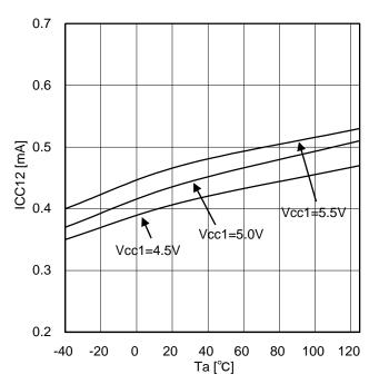
Figure 20. Input side circuit current (at OUT1=H)
