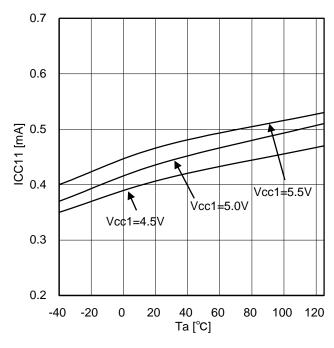
Figure 18. Input side circuit current (at OUT1=L)
