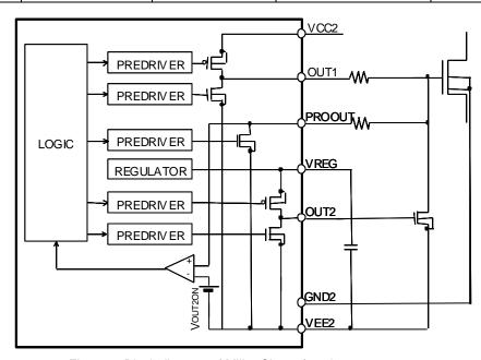
Figure 4. Block diagram of Miller Clamp function
