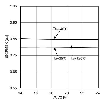
Figure 56. SCP detection mask time
