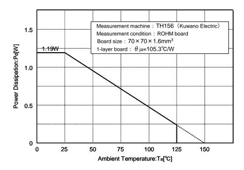
Figure 64. SSOP-B20W Derating Curve
