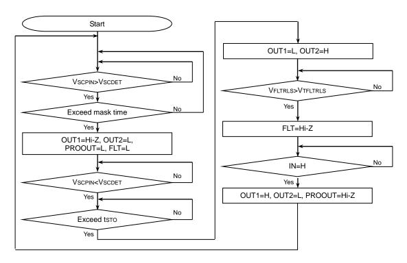
Figure 13. SCP Operation Status Transition Diagram
