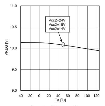
Figure 49. VREG output voltage
