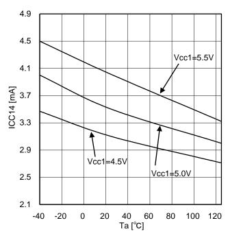
Figure 24. Input side circuit current (at INA=20kHz and Duty=50%)
