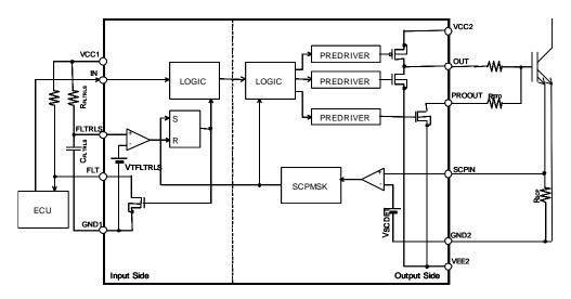
Figure 14. Block Diagram for SCP
