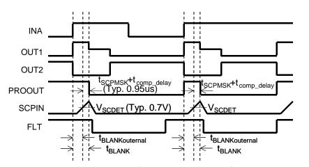
tcomp\_delay: Detection delay time of internal comparator
