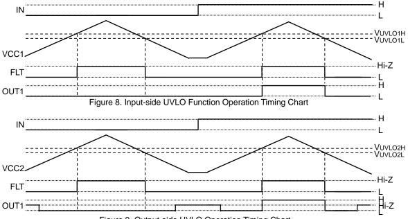
Figure 9. Output-side UVLO Operation Timing Chart
