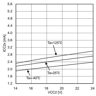
Figure 27. Output side circuit current (at OUT1=H)
