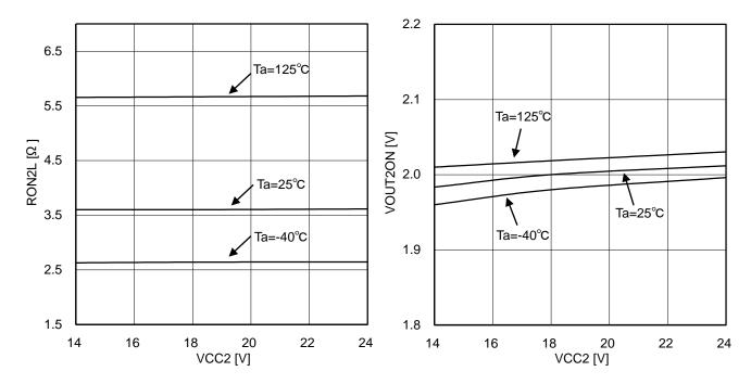
Figure 45. OUT2 ON resistance (Sink)
