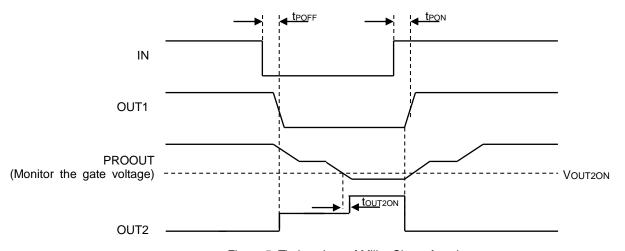
Figure 5. Timing chart of Miller Clamp function
