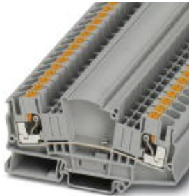
Feed-through terminal block, Connection method: Push-in connection, Cross section: 0.5 mm 2 -10 mm 2 , AWG: 20 - 10, Width: 8.2 mm, Color: gray
