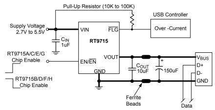
**Note**: A low-ESR 150uF aluminum electrolytic or tantalum between  $V_{OUT}$  and GND is strongly recommended to meet the 330mV maximum droop requirement in the hub  $V_{BUS}$ . (see Application Information Section for further details)
