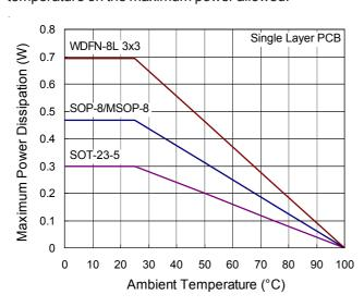
Figure 2. Derating Curves for RT9715 Package
