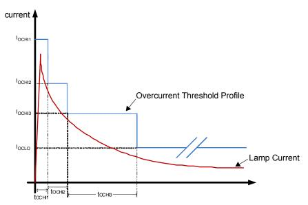
Figure 14. Transient overcurrent profile
