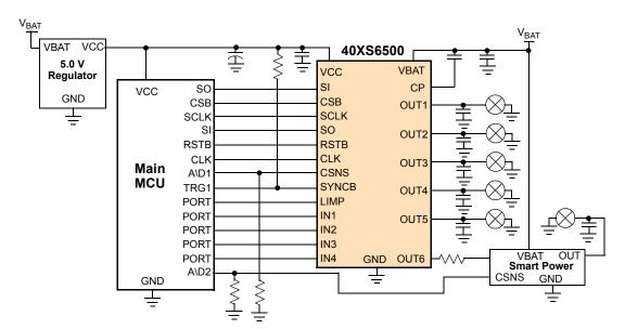
Figure 1. Penta 40 m $\Omega$  high-side simplified application diagram
