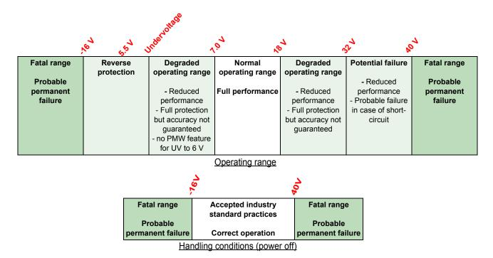
Figure 4. Ratings vs. operating requirements (VBAT pin)
