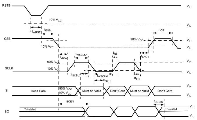
Figure 8. Timing requirements during SPI communication
