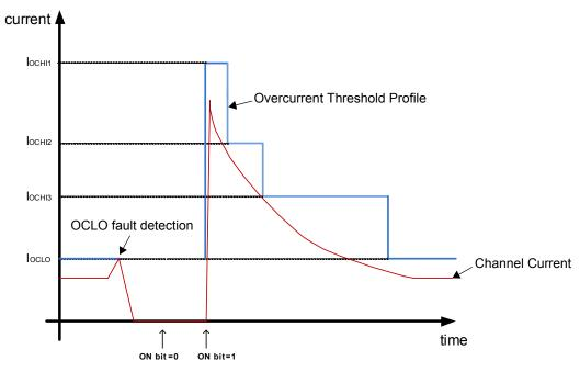
Figure 16. Resetable overcurrent profile
