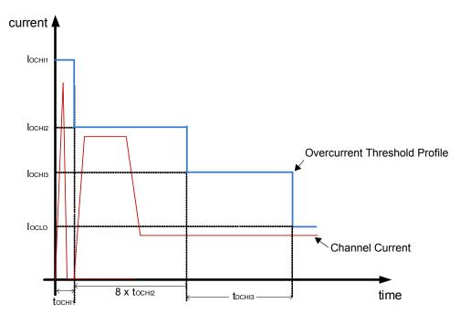
Figure 18. HID ballast overcurrent profile
