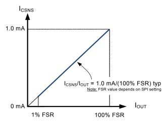
Figure 25. Output current sensing
