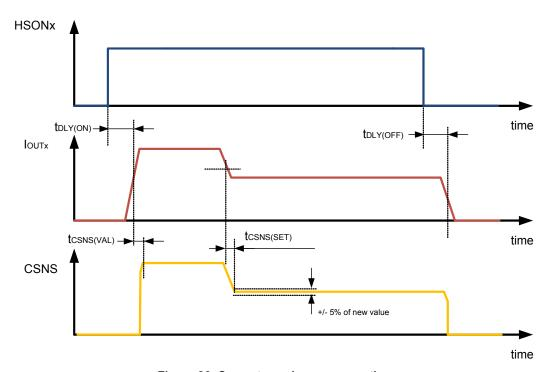
Figure 26. Current sensing response time
