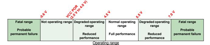
Figure 5. Ratings vs. operating requirements (VCC pin)
