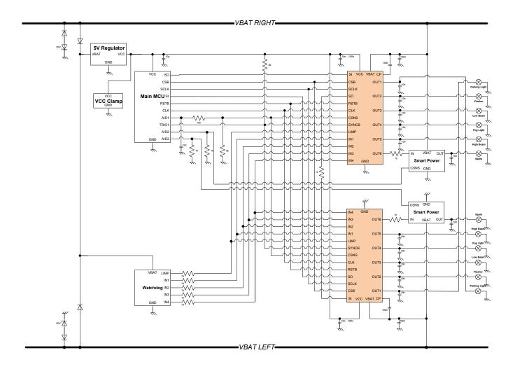
Figure 35. Typical automotive front lighting
