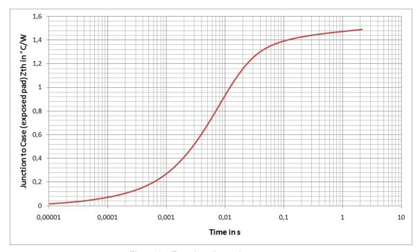
Figure 37. Transient thermal response curve
