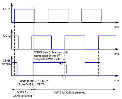
Figure 30. CSNS SYNCB TRIG0 setting
