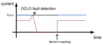
Figure 17. Overcurrent level fixed to OCLO
