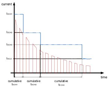
Figure 15. Transient overcurrent profile in PWM mode
