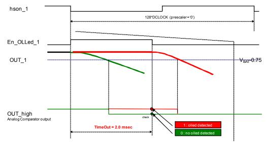
Figure 22. Open load in on state for LED in PWM operation (off-time > 2.0 ms)
