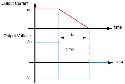
Figure 20. Simplified negative output clamp waveform
