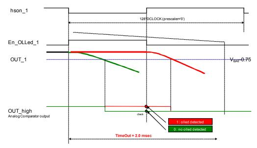
Figure 23. Open load in on state for LED in PWM operation (off-time < 2.0 ms)
