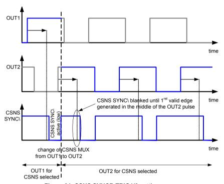
Figure 31. CSNS SYNCB TRIG1/2 setting
