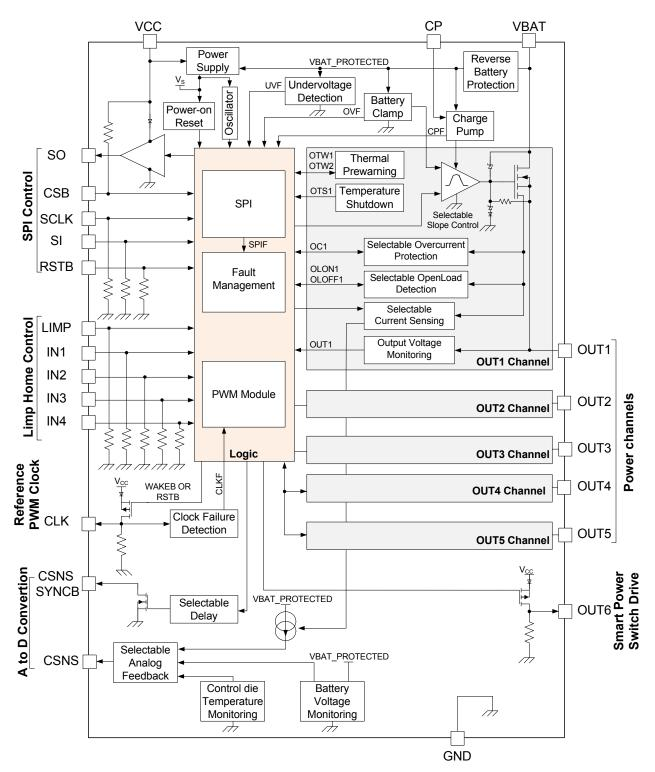
Figure 2. 12XS6 simplified internal block diagram (penta version)
