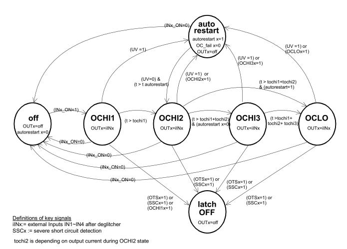
Figure 13. Output control diagram in fail mode
