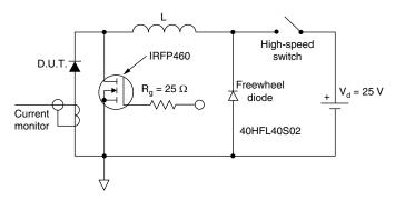
Fig. 8 - Unclamped Inductive Test Circuit
