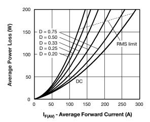
Fig. 6 - Forward Power Loss Characteristics
