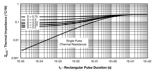
Fig. 4 - Maximum Thermal Impedance Z<sub>thJC</sub> Characteristics
