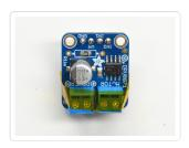
Solder in both pins of each terminal block. You can remove the tape when done.
