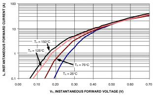
Figure 2. Typical Forward Characteristics, Per Element
