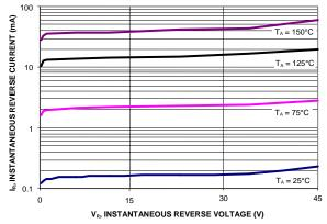
Figure 3. Typical Reverse Characteristics, Per Element
