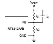
Figure 1. Cff Capacitor Setting
