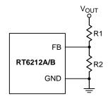
Figure 5. Output Voltage Setting
