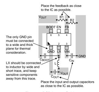
Figure 8. PCB Layout Guide
