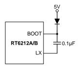
Figure 6. External Bootstrap Diode
