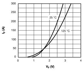
Fig. 9 - Diode Typical Forward Characteristics
