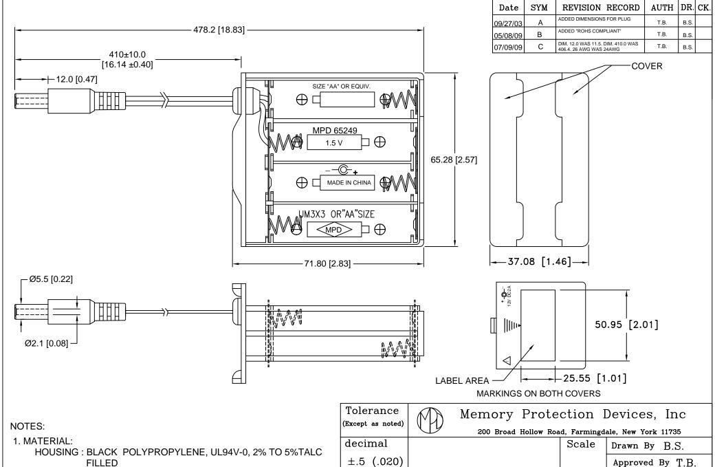
SPRING: SPRING STEEL, NICKLE PLATED CONTACTS: SPRING STEEL, NICKLE PLATED
