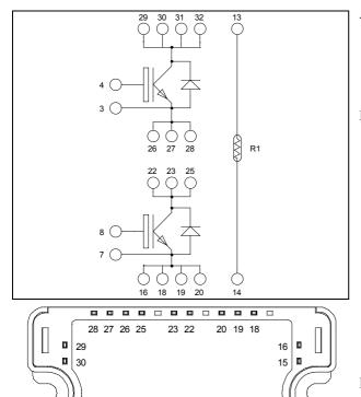
Pins 29/30/31/32 must be shorted together Pins 26/27/28/22/23/25 must be shorted together to achieve a phase leg Pins 16/18/19/20 must be shorted together
