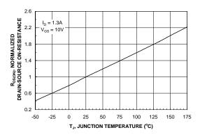
Figure 3. On-Resistance Variation with Temperature.
