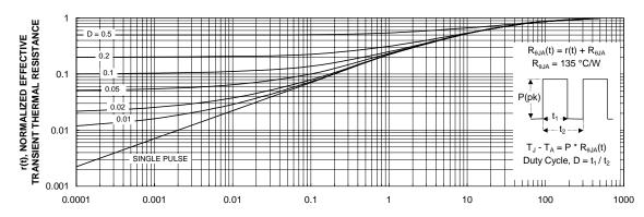
Figure 11. Transient Thermal Response Curve.
