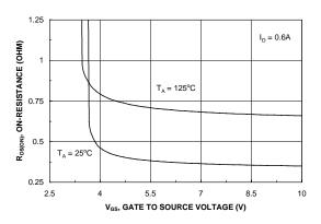
Figure 4. On-Resistance Variation with Gate-to-Source Voltage.
