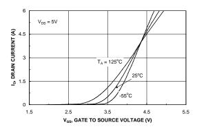
Figure 5. Transfer Characteristics.
