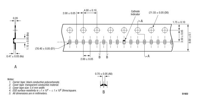
**Figure 4. SOD-882 Tape and Reel Dimensions**
