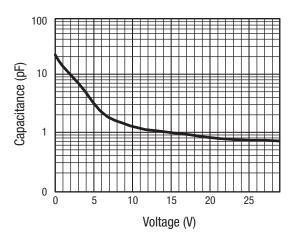
Figure 1. Capacitance vs Voltage @ 25 °C
