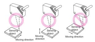
Install the Sensor as shown in the following illustration if each sensing object greatly differs in color or material.
