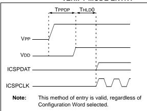
FIGURE 3-2: VDD-FIRST PROGRAM/ VERIFY MODE ENTRY
