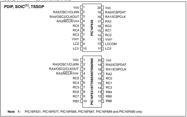
FIGURE 1-5: 20-PIN DIAGRAM FOR PIC16F631/677/685/687/689/690
