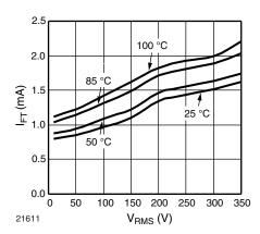
Fig. 7 - Trigger Current vs.
