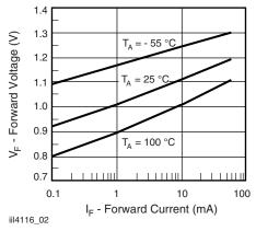
Fig. 2 - Forward Voltage vs. Forward Current
