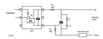
Fig. 12 - Basic Power Triac Driver Circuit
