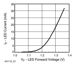
Fig. 1 - LED Forward Current vs. Forward Voltage
