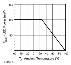
Fig. 4 - Maximum LED Power Dissipation
