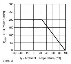
Fig. 6 - Maximum Output Power Dissipation
