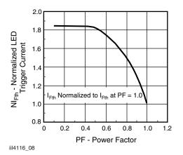
Fig. 10 - Normalized LED Trigger Current
