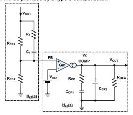
FIGURE 66. TYPE-3 COMPENSATOR
