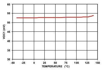
FIGURE 43. OC1 VOLTAGE THRESHOLD (ACROSS RSEN) vs TEMPERATURE
