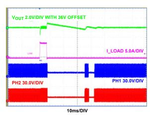
FIGURE 30. DE MODE (DE/PHDRP = VCC), TRANSIENT RESPONSE,  $I_{OUT}$  = 0.03A TO 8A STEP LOAD
