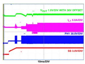
FIGURE 6. EN INTO PREBIASED OUTPUT, CCM MODE  $(\mbox{DE/PHDRP} = \mbox{GND}), \mbox{I}_{\mbox{OUT}} = \mbox{OA}$
