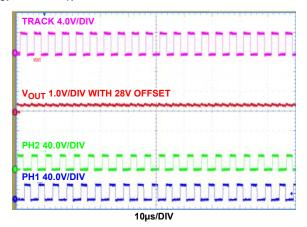
FIGURE 29. DIGITAL TRACKING, (TRACKING SIGNAL, FREQUENCY = 200kHz, D\_TRACK = 0.5), V<sub>OUT</sub> = 28.3V
