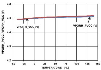
FIGURE 42. PVCC/VCC POR RISING THRESHOLD vs TEMPERATURE
