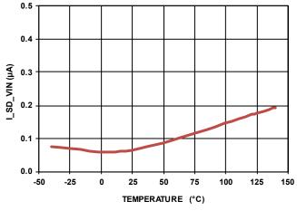
FIGURE 33. SHUTDOWN CURRENT AT THE VIN PIN I\_SD vs TEMPERATURE,  $V_{\rm IN} = 55 V$
