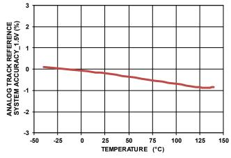
FIGURE 46. ANALOG TRACKING REFERENCE SYSTEM ACCURACY vs TEMPERATURE, MEASURED AT THE FB PIN, V<sub>TRACK</sub> = 1.5V
