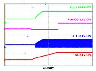
FIGURE 11. SOFT-START, DE MODE (DE/PHDRP = VCC), I<sub>OUT</sub> = 8A
