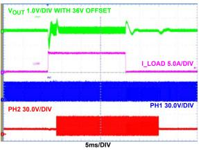
FIGURE 32. DE+PH\_DROP MODE (DE/PHDRP = FLOAT), TRANSIENT RESPONSE, I<sub>OUT</sub> = 1A TO 8A STEP LOAD
