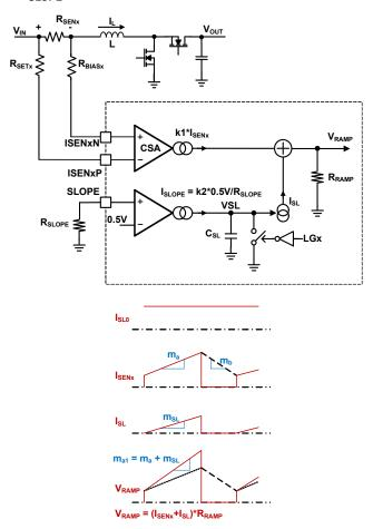
FIGURE 61. SLOPE COMPENSATION BLOCK DIAGRAM
