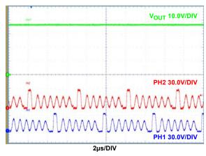
FIGURE 18. DE MODE (DE/PHDRP =  $V_{CC}$ ), DIODE EMULATION OPERATION, I<sub>OUT</sub> = 29mA
