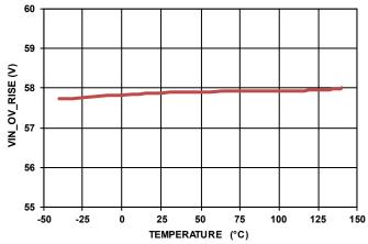
FIGURE 41. VIN OV RISING THRESHOLD VS TEMPERATURE
