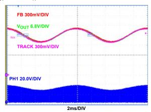
FIGURE 23. ANALOG TRACKING 100Hz SINUSOIDAL SIGNAL, CCM MODE (DE/PHDRP = GND), ATRK/DTRAK = VCC,  $I_{OLIT}$  = 1A
