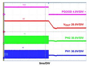
FIGURE 15. EN SHUTDOWN, I<sub>OUT</sub> = 8A
