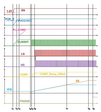
FIGURE 58. CIRCUIT INITIALIZATION AND SOFT-START
