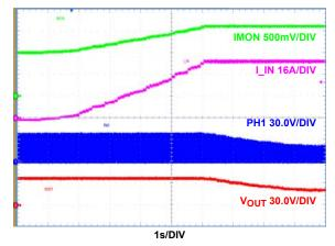
FIGURE 27. LOAD CURRENT KEEP INCREASING FROM NO LOAD TO OVERLOAD (25A), V<sub>OUT</sub> STARTS TO DROP WHEN INPUT CONSTANT CURRENT MODE STARTS TO WORK, INPUT CURRENT IS FINALLY CONTROLLED TO BE CONSTANT
