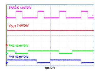
FIGURE 28. DIGITAL TRACKING (TRACKING SIGNAL, FREQUENCY = 400kHz, D\_TRACK = 0.3), V<sub>OUT</sub> = 17V
