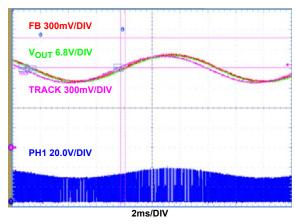
FIGURE 24. ANALOG TRACKING 300Hz SINUSOIDAL SIGNAL AT THE TRACK PIN, CCM MODE (DE/PHDRP = GND), ATRK/DTRAK = VCC, I<sub>OUT</sub> = 1A
