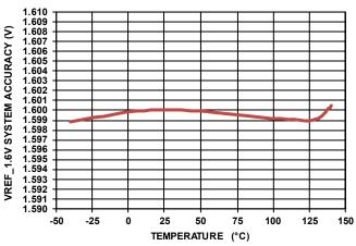
FIGURE 38. VREF 1.6V SYSTEM ACCURACY vs TEMPERATURE, **MEASURED AT THE FB PIN**
