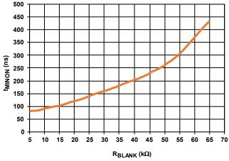
FIGURE 57. t<sub>MINON</sub> vs RBLANK
