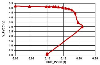
FIGURE 62. INTERNAL LDO OUTPUT VOLTAGE vs LOAD
