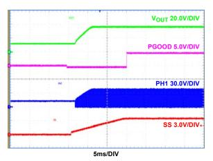
FIGURE 10. SOFT-START, DE+PHDROP MODE (DE/PHDRP = FLOAT),  $I_{OUT} = 8A$
