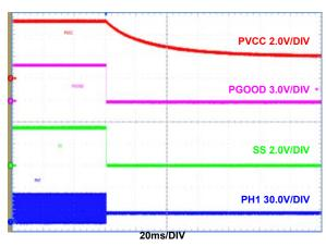
FIGURE 12. EN SHUTDOWN, PVCC/PGOOD/SS FALL,  $I_{OUT} = 0A$
