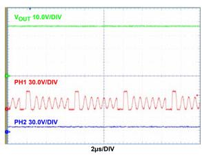
FIGURE 20. DE+PH DROP MODE (DE/PHDRP = FLOAT), PH1 DIODE EMULATION WITH PH2 DROPPED, I<sub>OUT</sub> = 29mA
