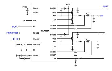
FIGURE 1. SIMPLIFIED APPLICATION SCHEMATIC, 2-PHASE SYNCHRONOUS BOOST
