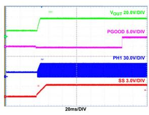
FIGURE 8. SOFT-START, CCM MODE (DE/PHDRP = GND),  $I_{OUT}$  = 8A
