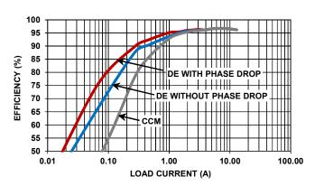
FIGURE 5. EFFICIENCY vs LOAD, 2-PHASE BOOST, 3 MODES OPERATION,  $f_{SW}$  = 200kHz,  $V_{IN}$  = 12V,  $V_{OUT}$  = 36V,  $T_A$  = +25°C
