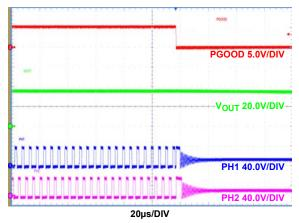
FIGURE 13. EN SHUTDOWN, I<sub>OUT</sub> = 8A
