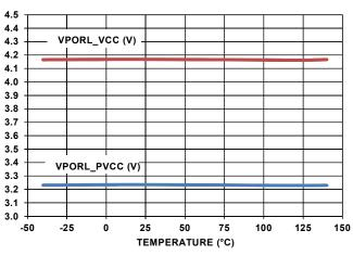
FIGURE 44. PVCC/VCC POR FALLING THRESHOLD vs TEMPERATURE
