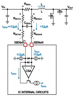
FIGURE 60. CURRENT-SENSING BLOCK DIAGRAM
