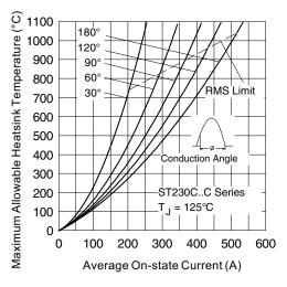
Fig. 5 - On-State Power Loss Characteristics
