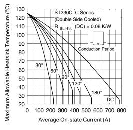
Fig. 4 - Current Ratings Characteristics
