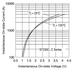
Fig. 9 - On-State Voltage Drop Characteristics
