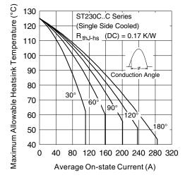
Fig. 1 - Current Ratings Characteristics
