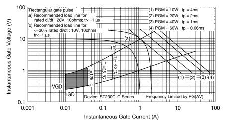
Fig. 11 - Gate Characteristics
