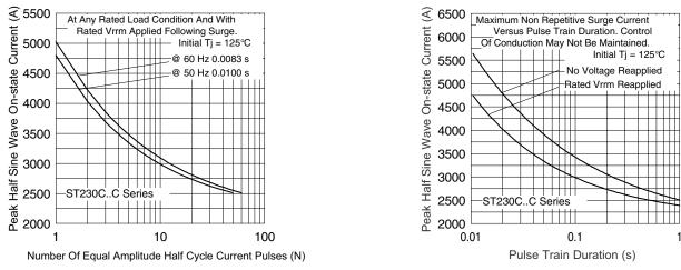
Fig. 7 - Maximum Non-Repetitive Surge Current Single and Double Side Cooled
