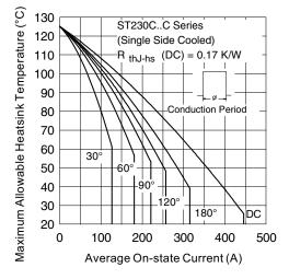
Fig. 2 - Current Ratings Characteristics
