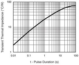
Fig. 6 - Typical Transient Thermal Impedance
