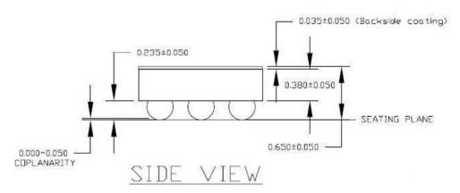
6-Bump, 0.5mm Pitch 1.5mm × 1.0mm Wafer Level Chip-Scale Package (CS)
