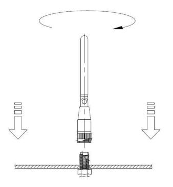
Recommended torque for mounting is 0.9 N-m Maximum torque for mounting is 1.176 N.m
