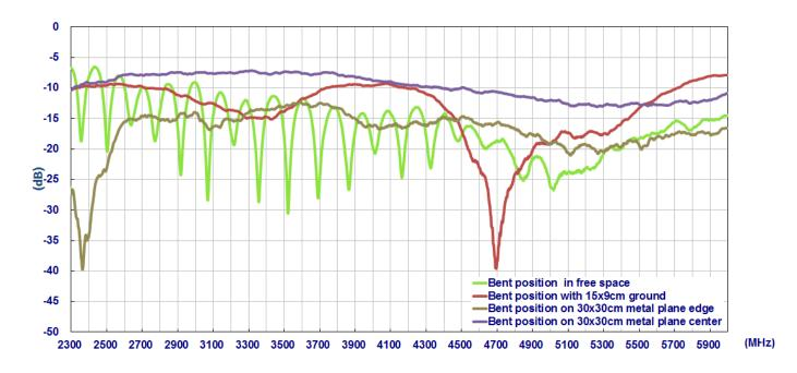
Figure3. Return loss of GW.05 antenna with bent position
