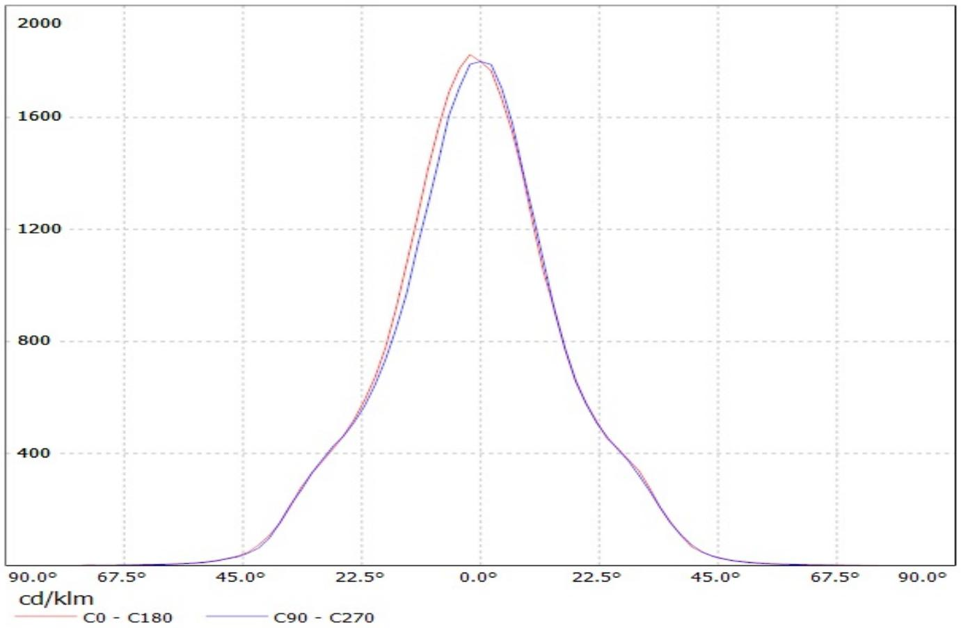
Luminaire: Ledil Oy CN12642\_LENINA-M-DL (Cree CXA20 698lm @ 250mA) Efficiency=77%
