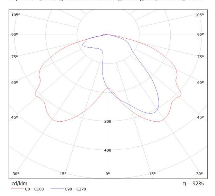
Luminaire: LEDiL Oy FCN14412\_STELLA-A\_(CXA1816) Lamps: 1 x Cree\_CXA1816\_844.151Im@250mA\_P=8.44487W\_I=249.9mA
