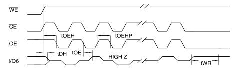
Notes: 1. Toggling either  $\overline{OE}$  or  $\overline{CE}$  or both  $\overline{OE}$  and  $\overline{CE}$  will operate toggle bit. The t<sub>OEHP</sub> specification must be met by the toggling input(s).
