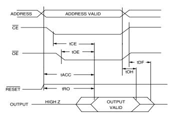
Notes: 1.  $\overline{\text{CE}}$  may be delayed up to  $t_{\text{ACC}}$  -  $t_{\text{CE}}$  after the address transition without impact on  $t_{\text{ACC}}$ .
