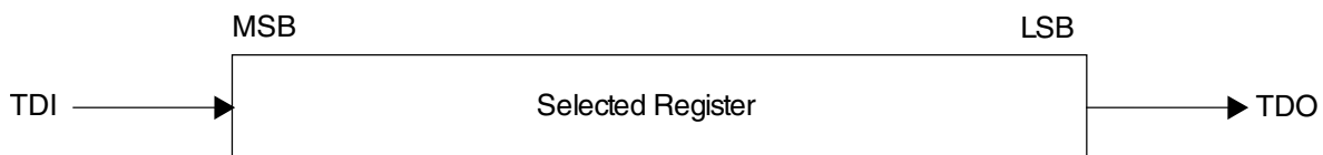
Figure 5-3. Shifting data through a register
