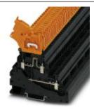
Disconnect terminal block, Connection type: Screw connection, Cross section: 0.14 mm² - 4 mm², AWG: 26 - 10, Nominal current: 28 A, Nominal voltage: 500 V, Length: 92.7 mm, Width: 6.2 mm, Color: black, Assembly: NS 35/7,5, NS 35/15
