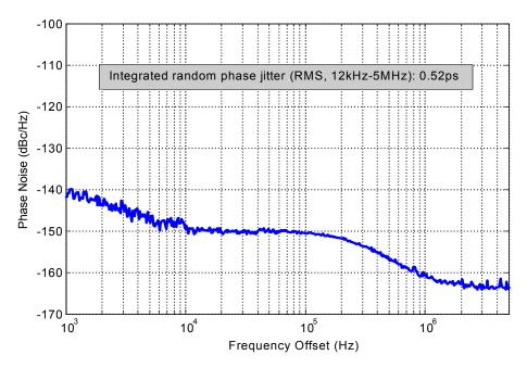
Figure 3. Phase Noise, 10 MHz, 3.3V, LVCMOS Output
