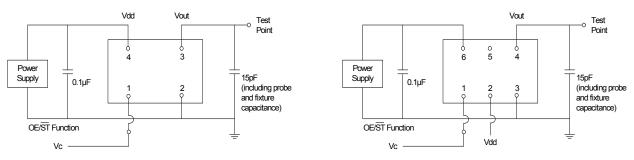
Figure 4. Test Circuit (4-Pin Device)
