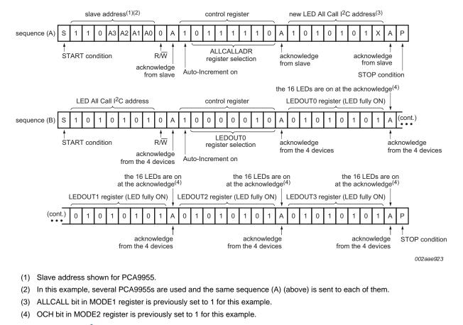
Fig 19. LED All Call I<sup>2</sup>C-bus address programming and LED All Call sequence example
