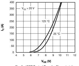
Fig. 2 - IGBT Typical Transfer Characteristics
