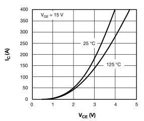
Fig. 1 - IGBT Typical Output Characteristics
