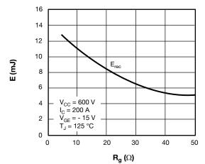
Fig. 9 - Diode Switching Loss vs. Gate Resistance
