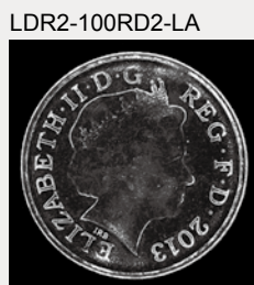
LDR2-100RD2-LA Illuminating from a low angle allows for imaging that emphasizes the edges.
