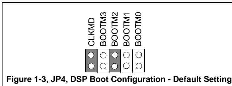
**Figure 1-3, JP4, DSP Boot Configuration - Default Setting**
