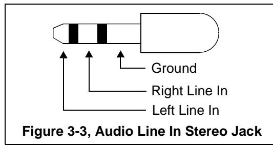
Figure 3-3, Audio Line In Stereo Jack
