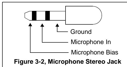
Figure 3-2, Microphone Stereo Jack
