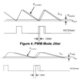
Figure 5: Skip-Mode Jitter Ramp with a Large ESR Capacitor
