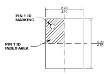
16-Pin QFN (3×4mm)
