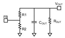
Figure 8: Simplified Skip-Mode Circuit
