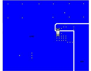
Figure 14: Bottom Layer, 13-Pin PFN MP8761 PCB Layout Guide
