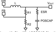
Figure 10: Simplified POSCAP Circuit
