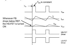
Figure 2: Heavy-Load Operation
