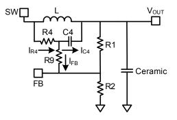
Figure 7: Simplified PWM-Mode Circuit with External Ramp Compensation
